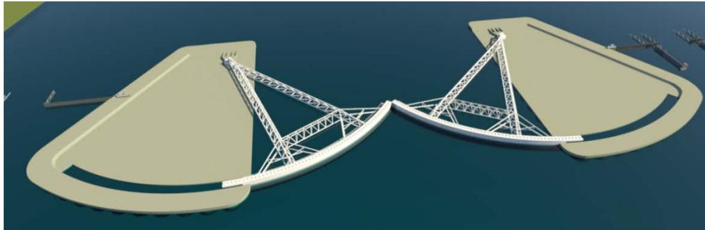
Figure 8: Floating Sector Gate and Artificial Island
