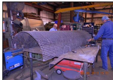
Scale Model of Breakwater Frame
