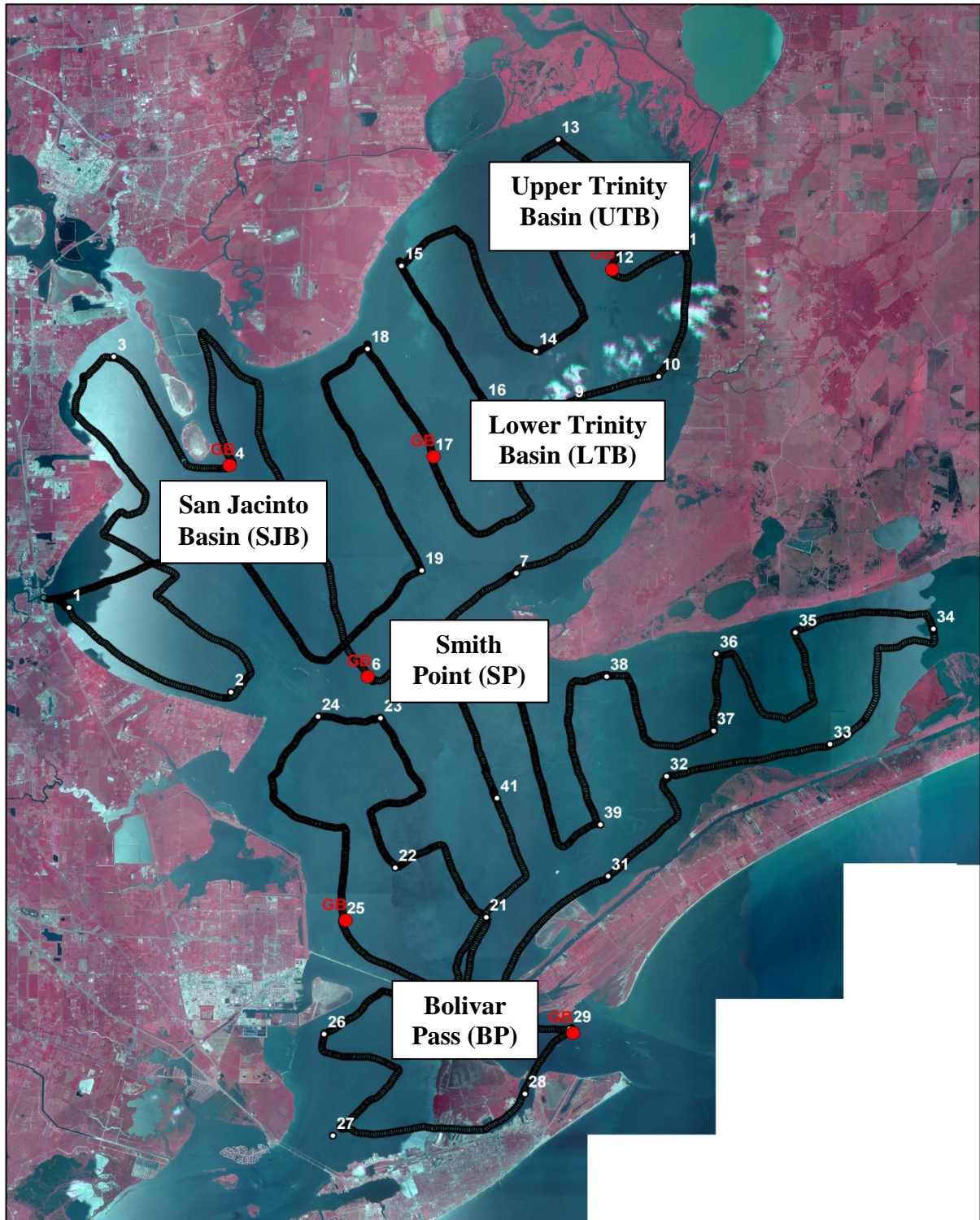
Fig. 1 Galveston Bay water quality parameters were examined along a tightly gridded transect shown by the black line. The northern part of the bay would typically take a day to complete, and the southern part a second day. Six fixed stations were sampled in order to check the calibration on the Dataflow. Ancillary measurements were also collected at stations in red as part of this project.
