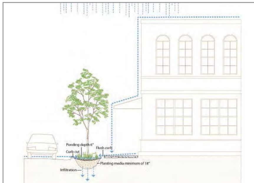
Figure 6-10: Schematic of a bioretention area with no underdrain creating a buffer between the pedestrian zone and the street; stormwater infiltrates into surrounding soils.
