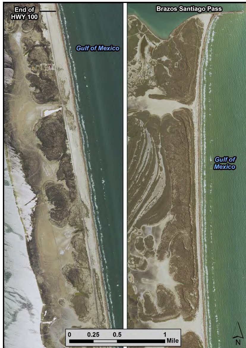
Figure 22 Oval-shaped characteristics of dune fields separated by overwash channels north (Left image) and south (right image) of Brazos Santiago Pass
