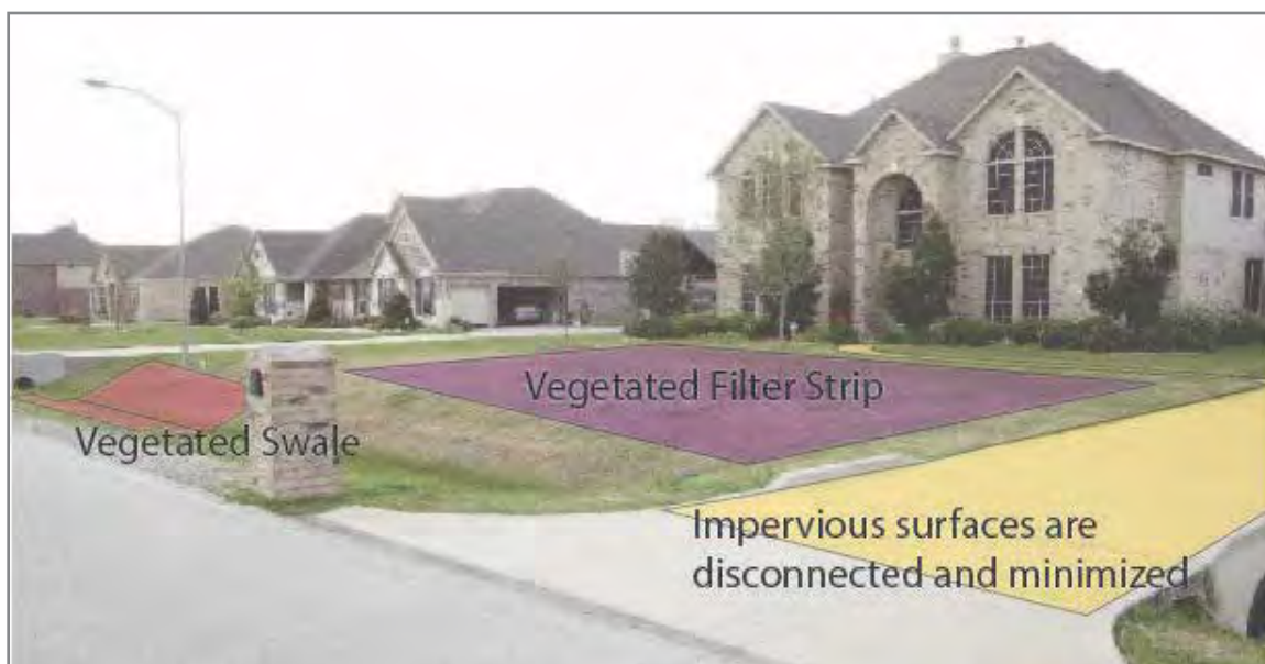
Figure 4-2: Medium density neighborhood uses vegetated swales for stormwater conveyance. These swales also provide water quality benefits.
