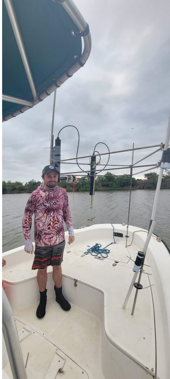
Figure 15: K. Capistrant-Fossa on a boat next to a prototype version of the eddy covariance frame. It has an acoustic doppler velocimeter and high-speed oxygen sensor in the center. Additional sensors for dissolved oxygen and irradiance are attached to the side.
