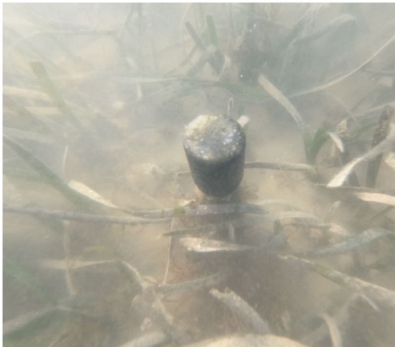
Figure 9: In-situ photographs of the acoustic source (top panel) and receiver (bottom panel) at East Flats. Biofouling required them to be gently wiped by hand in the field every few months.
