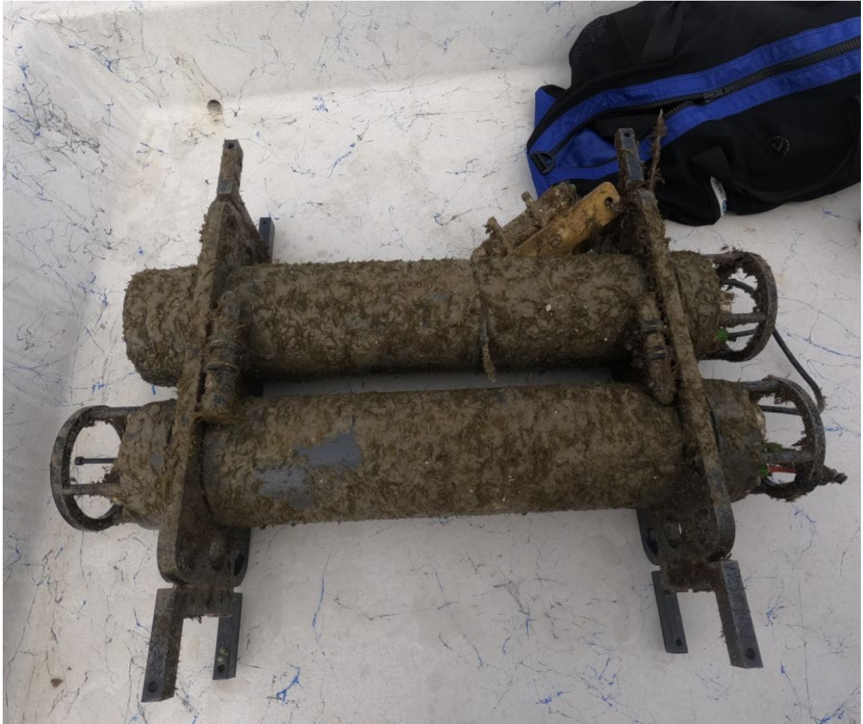
Figure 10: The electronic pressure housing from the acoustic array after recovery during a service trip. Tasks included cleaning, data downloading, and battery replacement.
