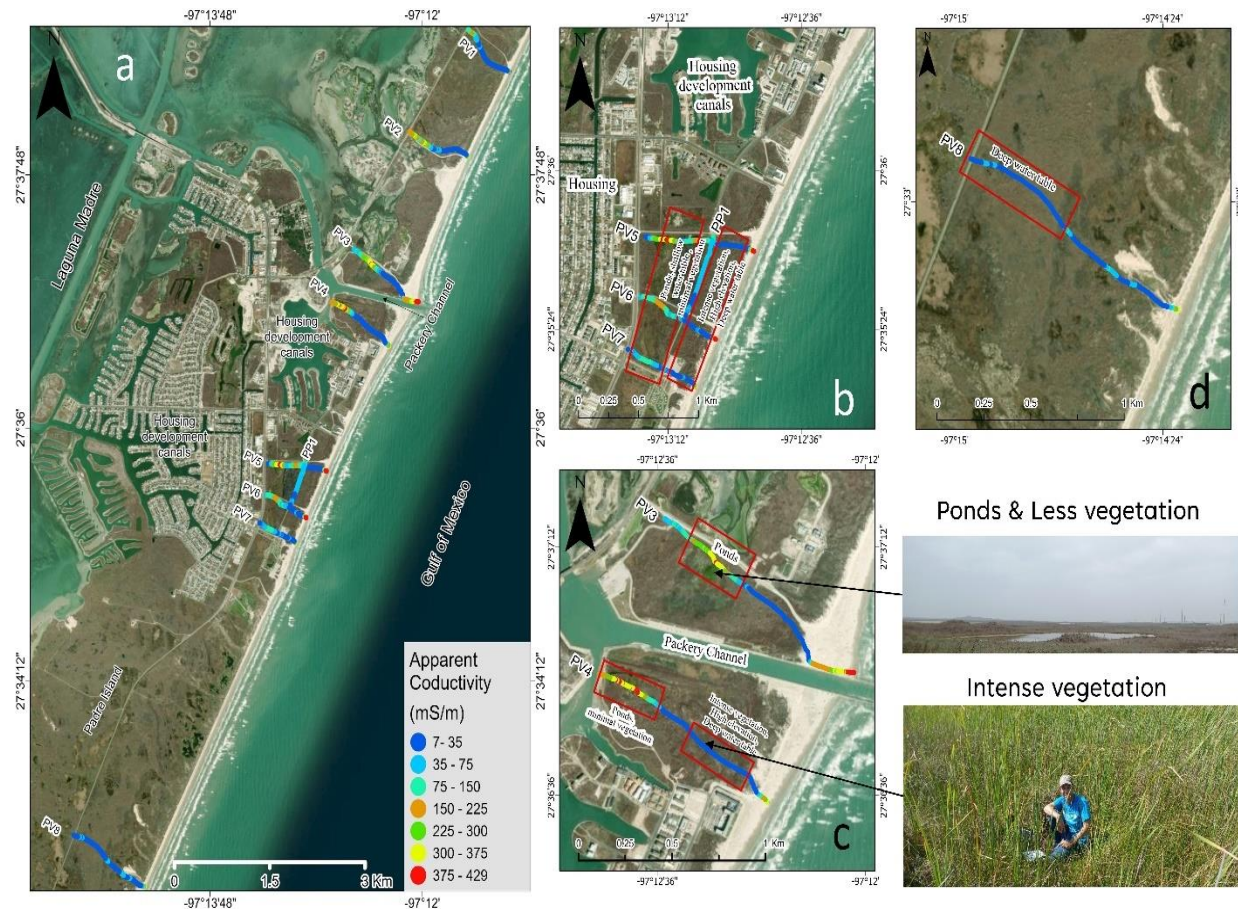
Figure 1- 3. (a) Island-wide distribution of apparent electrical conductivity across Padre Island. Panels (b), (c), and (d) relate those conductivity values to three surface variables: (b) the intensity of human development, (c) depth to the water table, and (d) vegetation cover (Abdelrehim et al., 2023).
