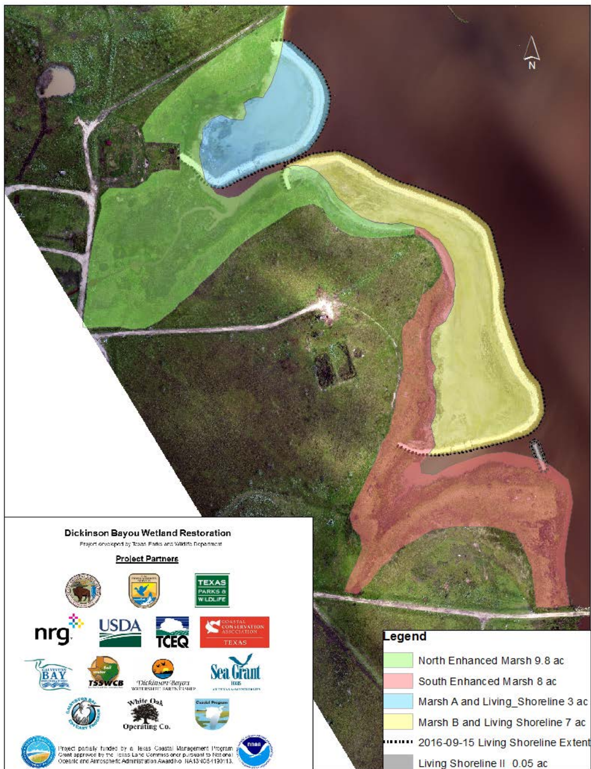
Figure 2. Final Post Construction Aerial Photograph taken by Naismith Surveying August 2016, with GIS based overlay showing created Marsh A and B and associated Living shoreline acreage (10 acres) and enhanced north and south marshes associated with adjacent tributaries (17.8 acres). The three living shorelines footprints were calculated by HDR from Naismith Survey. The enhanced north and south marsh acreage is based on GLO Coastal Boundary Survey and TPWD's wetland survey conducted in 2009.
