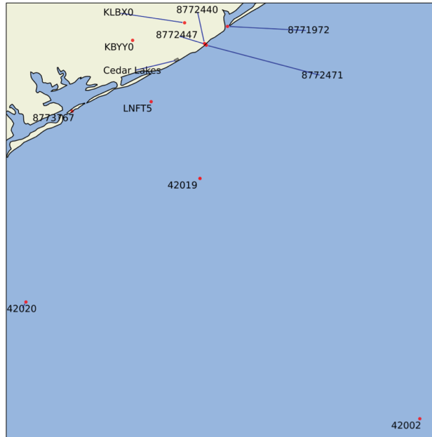
Figure 4: Locations of deep-water wave buoys, tidal gauge stations, and weather stations near Cedar Lakes.
