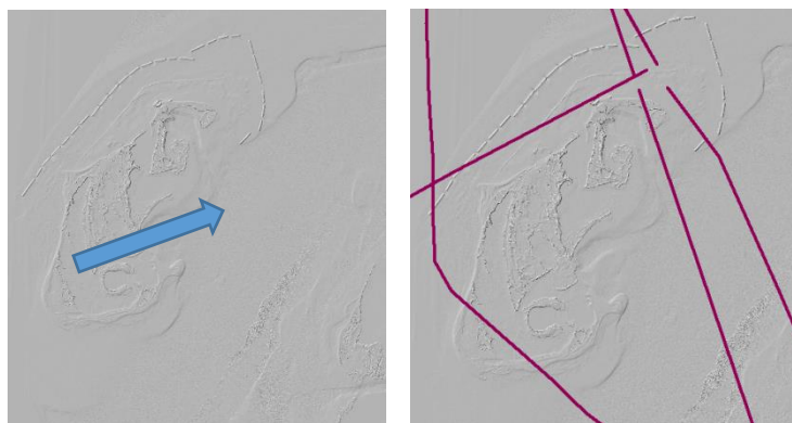
Figure 21. (left) Results of IDW interpolation shows only one major pipeline in the shaded relief DEM. (right) GLO shapefile is overlaid on the shaded relief as ground truth.
