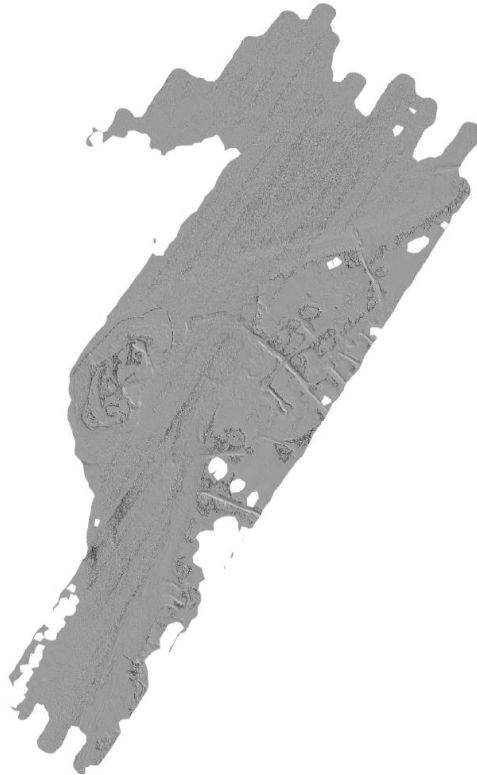
Figure 8. Shaded relief of a topo-bathymetric DEM at Shamrock Cove generated by fusing the “good” lidar data with the turbid water enhancement data over the data gap zone. Results show limited to no bottom detection.
