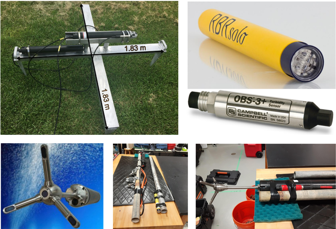
Figure 4.1: Top row - Aquadopp ADCP / OBS bottom-mounted frame, RBRsolo PT, and OBS-3+ sensor. Bottom row - Norkek Vector ADV and mounting pole.
