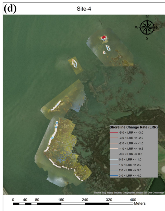
Figure 3.10: Graphical representation of the cumulative shoreline change rates in LRR at (a) FS-1, (b) FS-2, (c) FS-3, and (d) FS-4.
