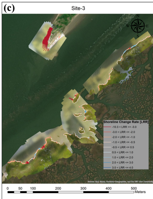
Figure 3.10: Graphical representation of the cumulative shoreline change rates in LRR at (a) FS-1, (b) FS-2, (c) FS-3, and (d) FS-4.
