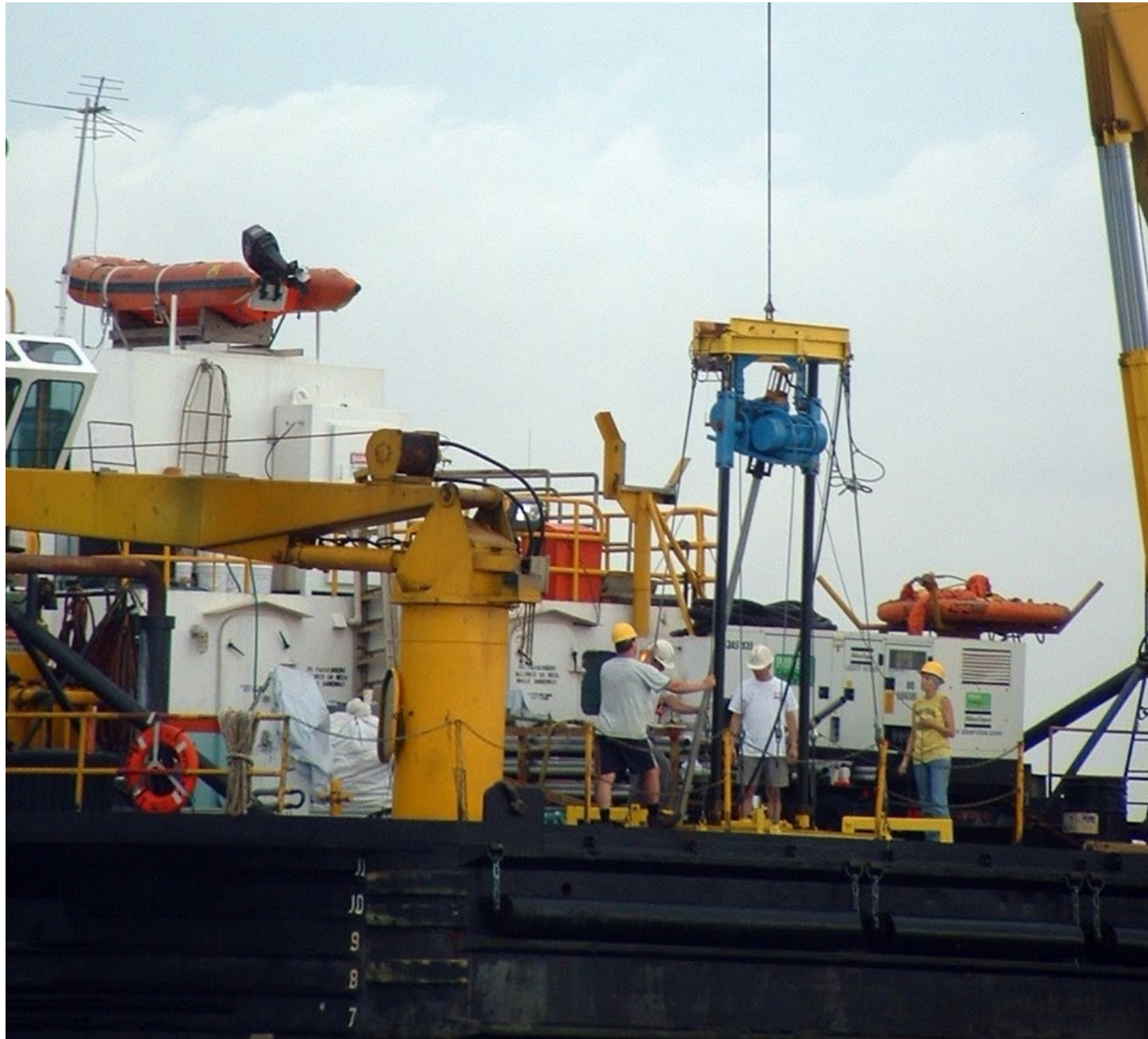
The deck of Lift Boat Ponthchatrain rigged with a submersible vibra core rig, the crew is rigging new core barrel.
