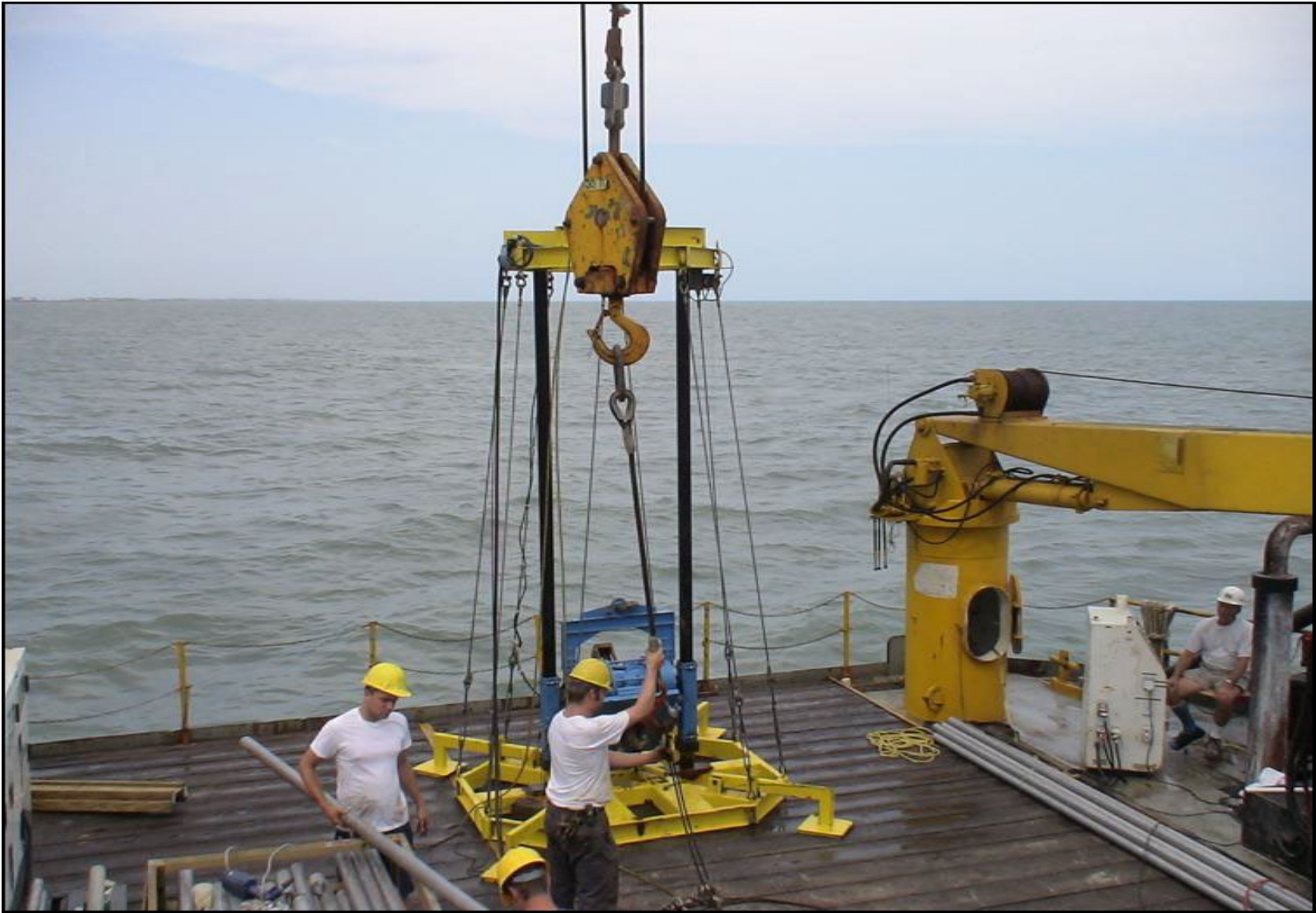
The deck of Lift Boat Ponthchatrain rigged with a submersible vibro core rig, the crew is rigging new core barrel.
