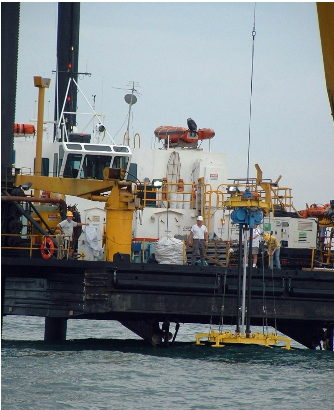
The deck of Lift Boat Ponthchatrain rigged with a submersible vibra core rig being deployed for core acquisition.
