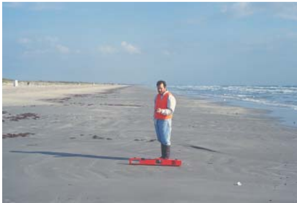
Figure 4. Topographically low, regularly flooded forebeach and higher irregularly flooded backbeach, MISP transect (waypoint 112). The conductivity meter (Geonics EM38) used to measure apparent ground conductivity is shown on the beach.
