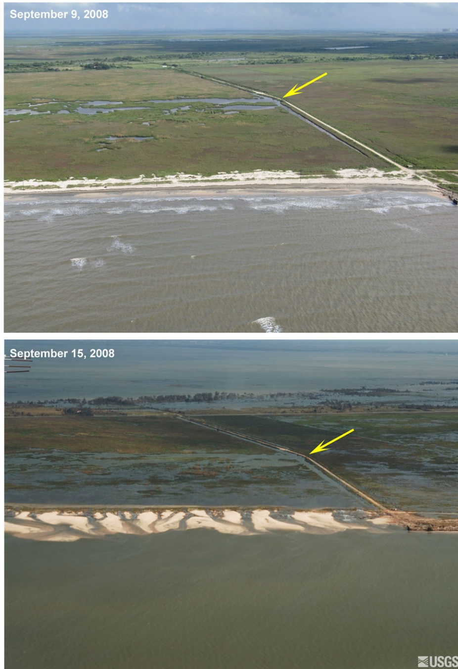
Figure 1.7. “Oblique aerial photography near the Texas Point National Wildlife Refuge, TX, on September 9, 2008 (top) and September 15, 2008, two days after landfall of Hurricane Ike (bottom). Yellow arrows mark features that appear in each image. Severe inundation and erosion of channels through the beach from a seaward-directed flow are evident here. http://coastal.er.usgs.gov/hurricanes/ike/photo-comparisons/highisland.html
