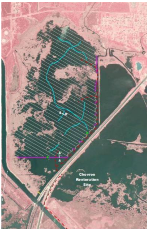
Figure 4: Hashed area depicts the area where dredge material was placed for the beneficial uses marsh along Highway 73 in Port Arthur, TX. The “Chevron Restoration Site” is the location of the engineered marsh described above.
