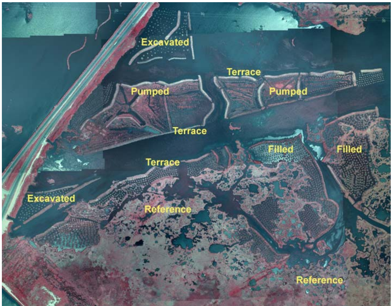
Figure 2: Aerial view of wetland restoration site in the Lower Neches Wildlife Management Area, taken September 2009. Areas of excavated, filled, and pumped mounds are noted; each mound area is surrounded by terraces. The reference site is located south of the constructed area.
