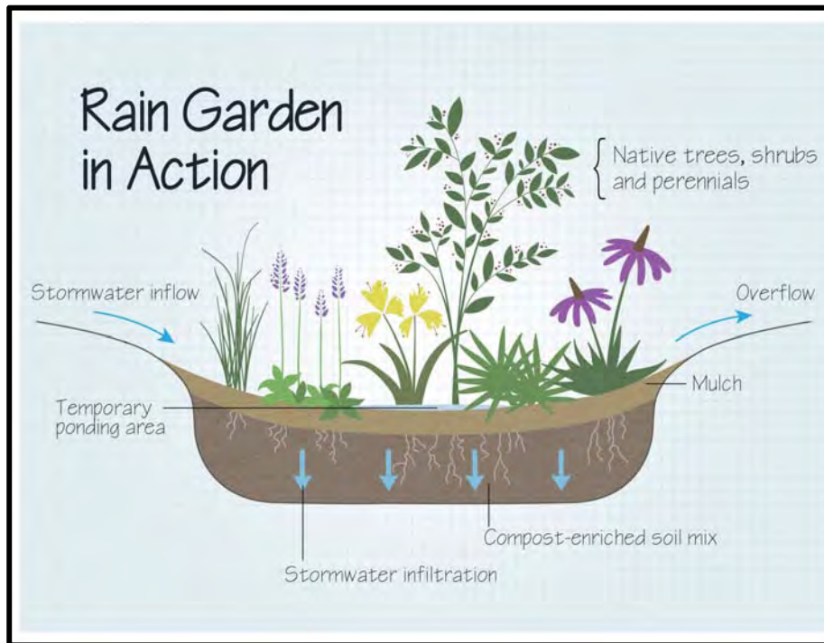
Graphic shows rain garden with no under drain
