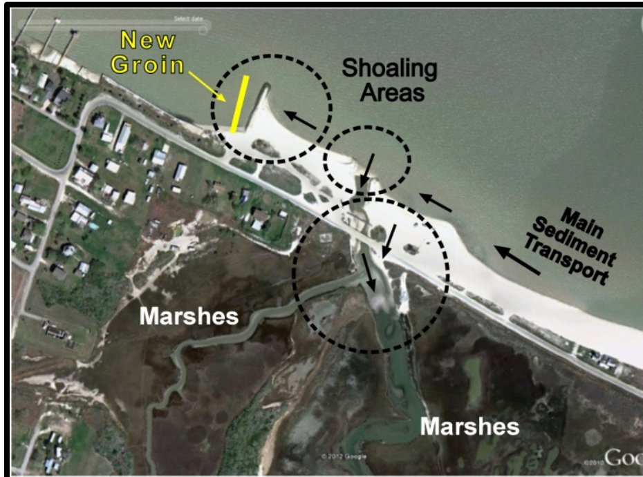
Figure B18. Shoaling areas in Magnolia next to the inlet channels connecting Matagorda Lavaca Bay with Old Town Lake.
