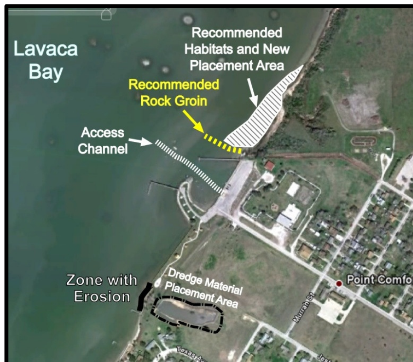
Figure B19. Potential BUDM opportunities and improvements to the boat ramp area, where dredged sediments could be used for the creation of marshes.
