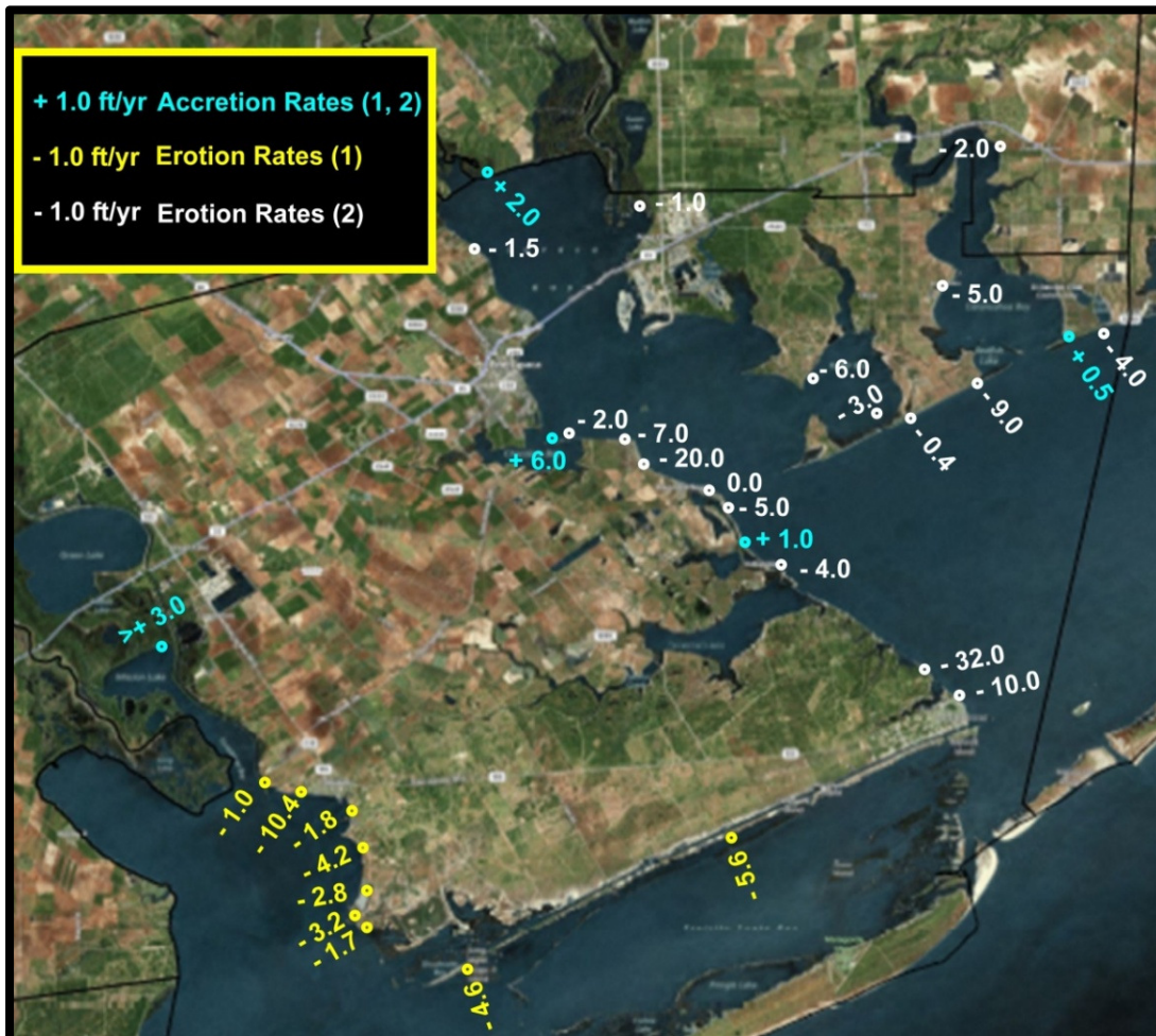
Figure B4. Erosion and accretion rates in ft/yr.
