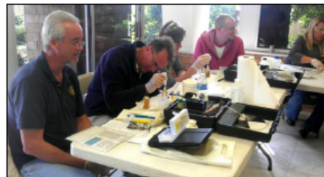
Doug Hughes & Mike Shebester (Sea Lake Yachts) & Kristian Rogers, Joshua Gunn & Erika Watson (GBF volunteers & staff) carry out tests to measure dissolved oxygen levels in water samples from Clear Lake.
