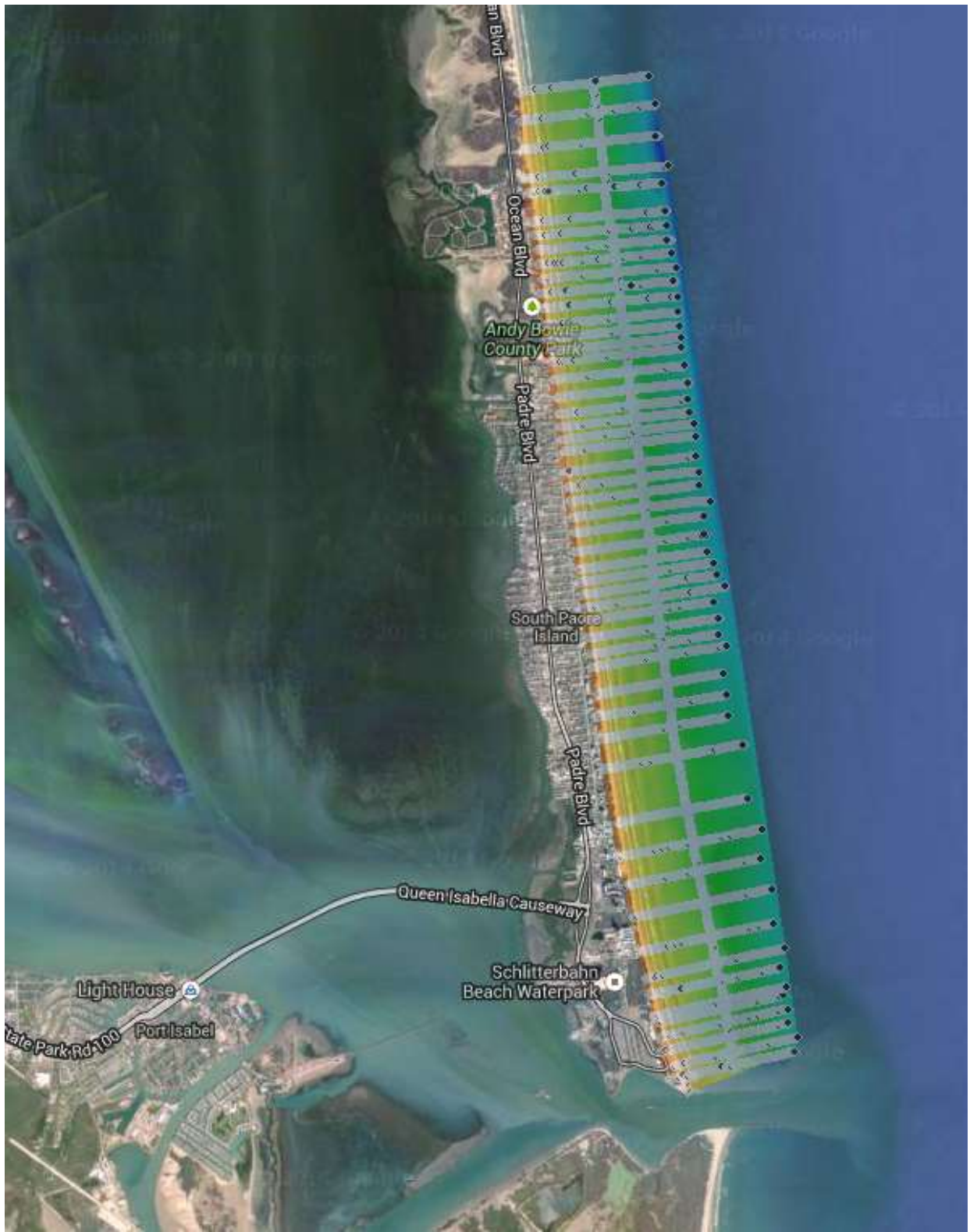
Figure 31. Single-beam sonar lines collected October 2012. Data from Naismith Marine Services, Inc.
