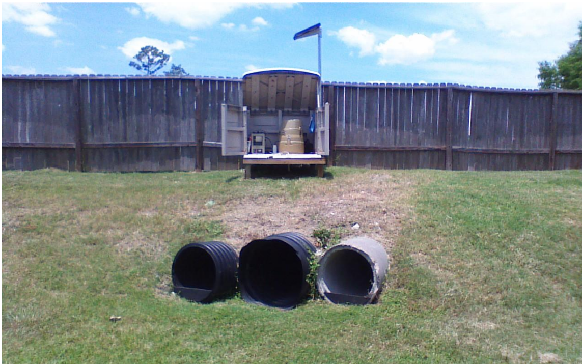
Figure 7. Detention basin used to collect runoff from the control site. All instrumentation is kept inside of a storage box on the apex of the basin.
