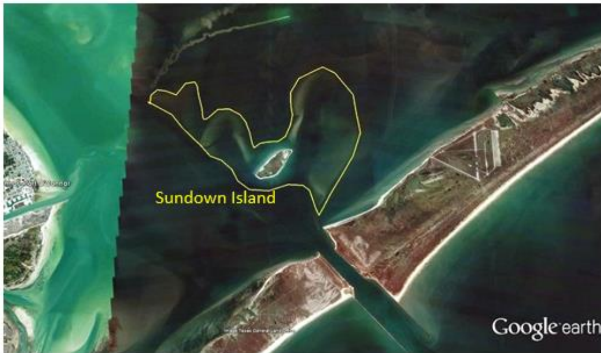
Figure 5-17, Location of the new sand bank created north of Sundown Island as result of the stronger tidal prism coming from the Gulf of Mexico through the Matagorda Ship Channel inlet.
