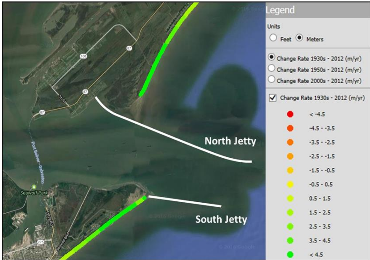
Figure 10-12, Galveston Ship Channel Entrance – Shoreline change Rate (BEG, 2016)
