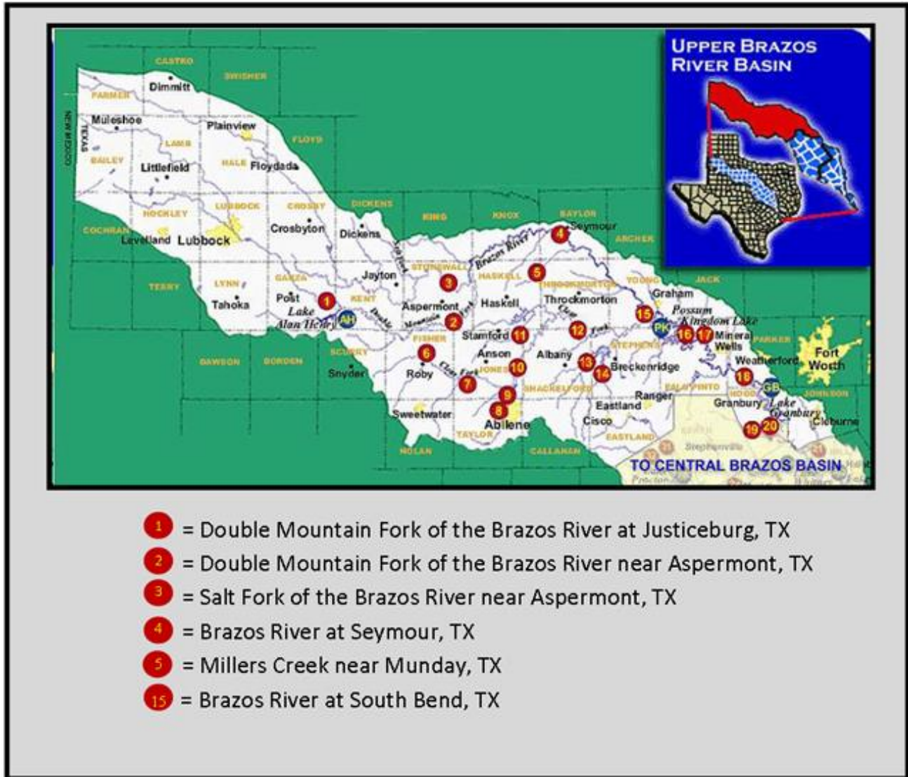
Figure 8-8, Upper Brazos River Map showing the Positions of the 6 USGS Gaging Station (Black, 2006).
