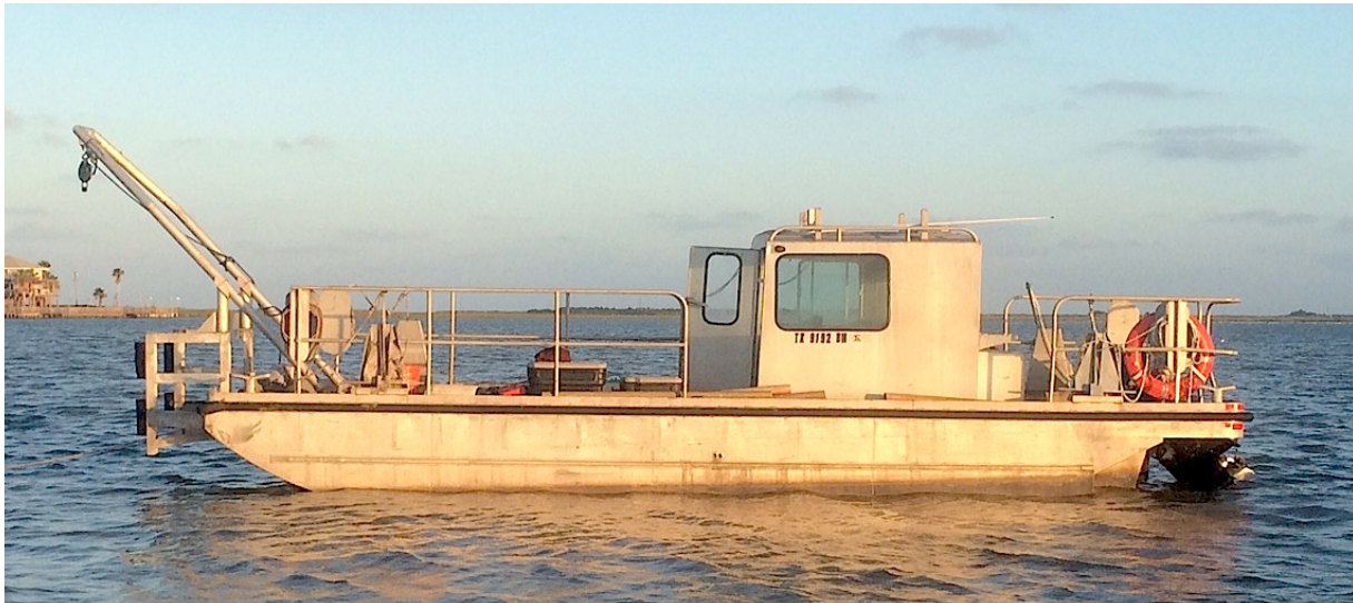
Figure 6.4. The R/V Big Daddy, TAMUG's 30 foot long motorized coring barge.
