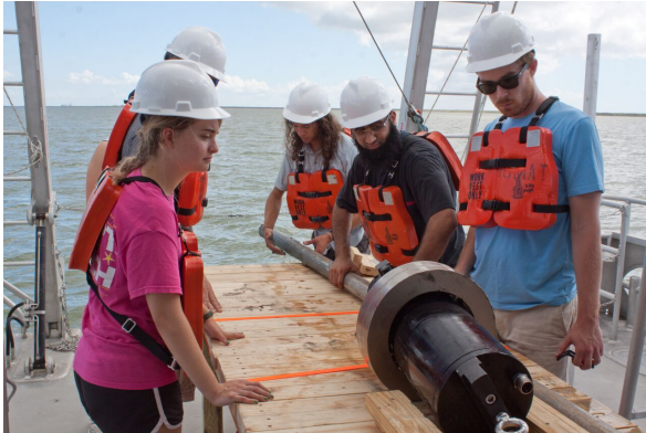
Figure 6.6. PVL-Tech vibra coring head on work bench while students mount core barrel to it.
