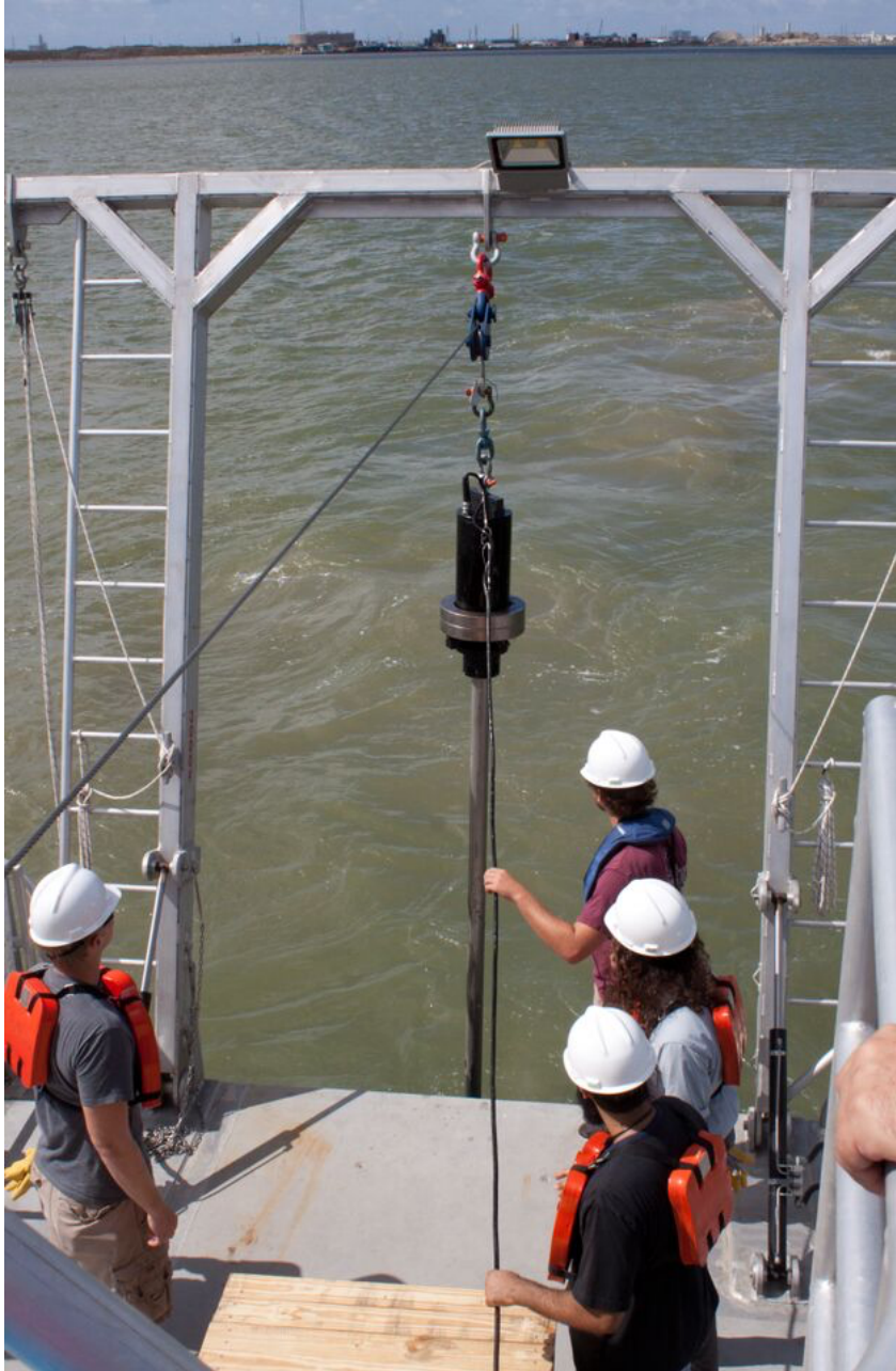
Figure 6.5. PVLI-Tech hanging from A-Frame aboard the R/V Trident, being tested on July 14.
