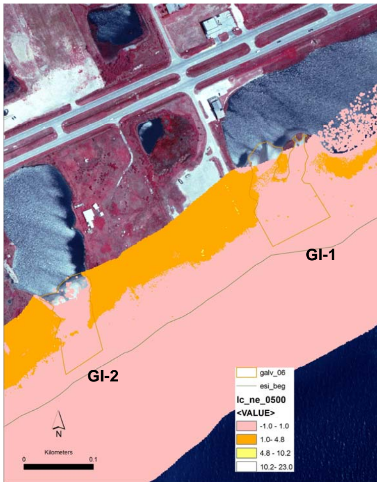
Figure 10. LIDAR elevations in meters (NAVD 88) correlate with unvegetated washover areas (yellow-lined polygon) identified from aerial photography.
