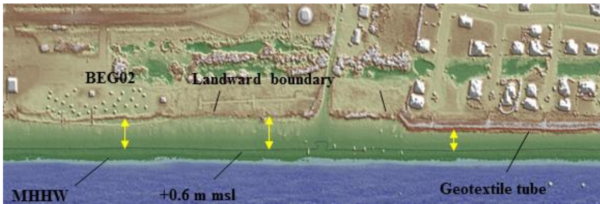
Figure 10. Lidar topographic-relief image of Galveston Island State Park and Pirates Beach subdivision. Note the difference in beach width between the natural beach and the area in front of the subdivision. From Gibeaut and others (2003).
