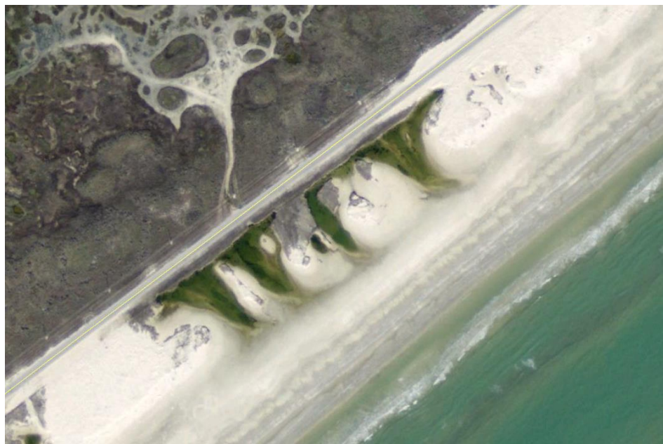
Figure 5.22 Vertical Aerial in 2009 (Google Earth) of area in vicinity of Monument B26. Note erosion of dune and scour areas along Bluewater Highway.
