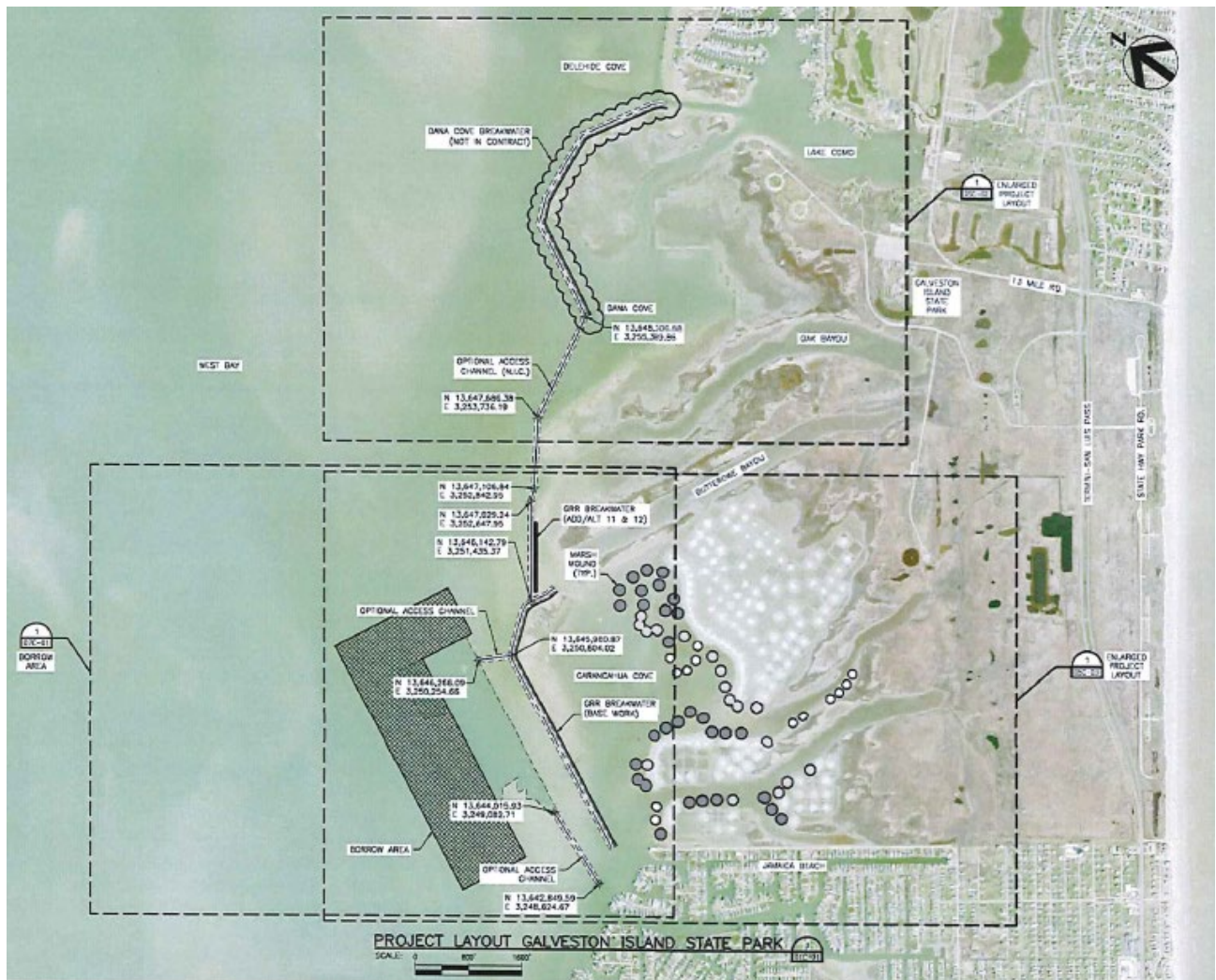
Figure 4.5.2 Project #1601 Plan View Drawing (Detail from HDR project record drawing dated April 2016)
