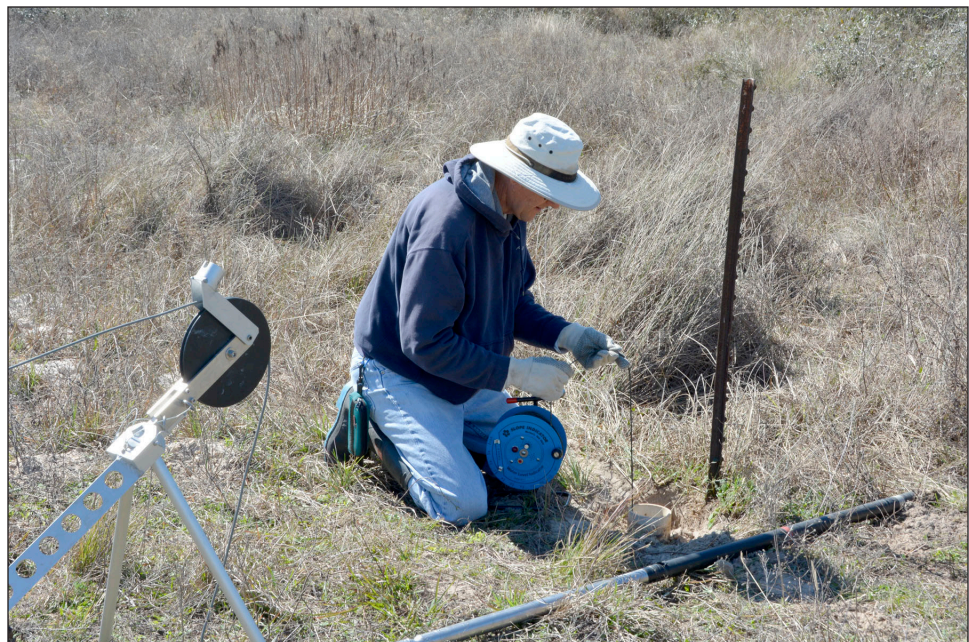
Figure 8. Measuring water depth in a PVC-cased water well before geophysical logging.
