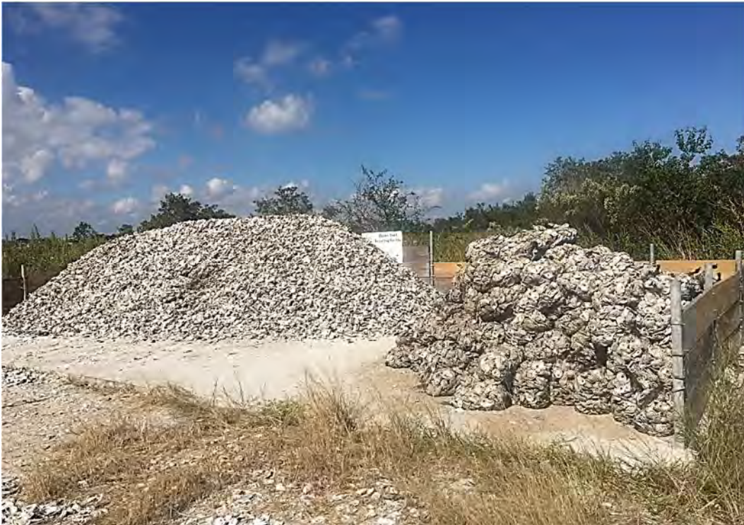
Figure 16. Newly piled shell and bagged shell at TX City Curing Site.
