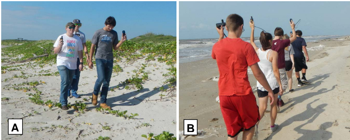
Figure 3. Students mapping (A) the vegetation line and (B) shoreline (wet/dry line) using handheld GPS units.
