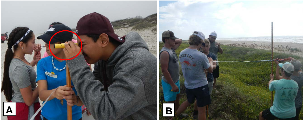
Figure 2. Students using (A) a sighting level to determine vertical offset between Emery rods, and (B) a metric tape to measure horizontal distance.
