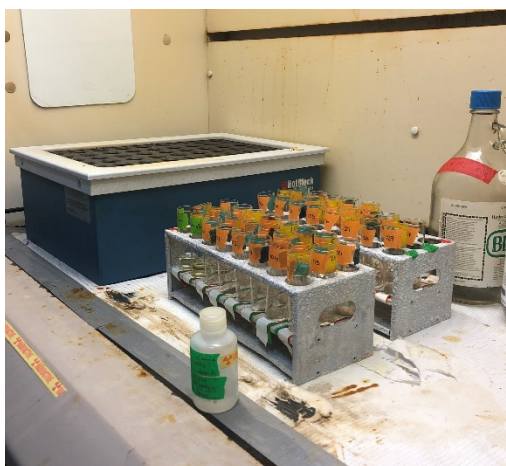
339 Figure 7: Hotblock used for acid digestion method for low ^{210}\text{Pb} activity samples
