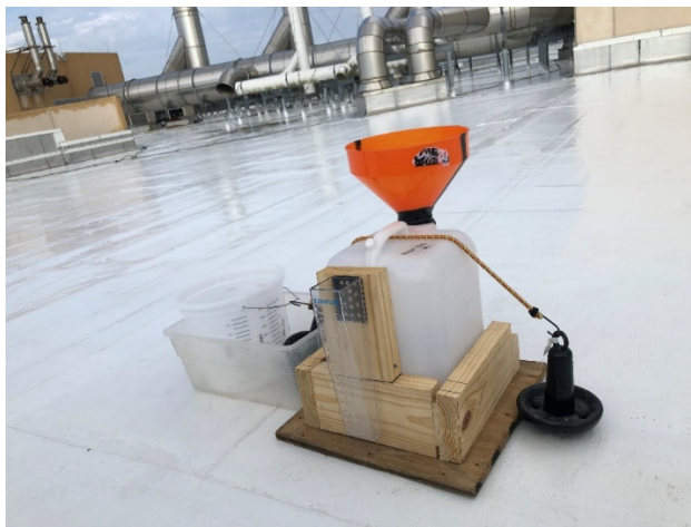
Figure 6: Precipitation jug with attachments mounted on the roof of OCSB located at Texas A&M University at Galveston.
