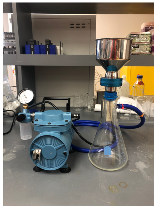
Figure 2. A) Van Dorn Sampler, used for collecting water samples at depth. B) Filtering apparatus used to vacuum filter water samples through a 0.45 \mu\text{m} gridded membrane filter
