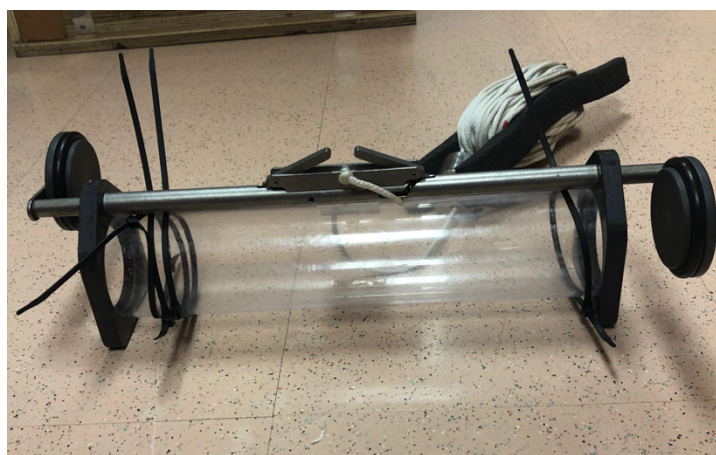
Figure 2. A) Van Dorn Sampler, used for collecting water samples at depth. B) Filtering apparatus used to vacuum filter water samples through a 0.45 \mu\text{m} gridded membrane filter
