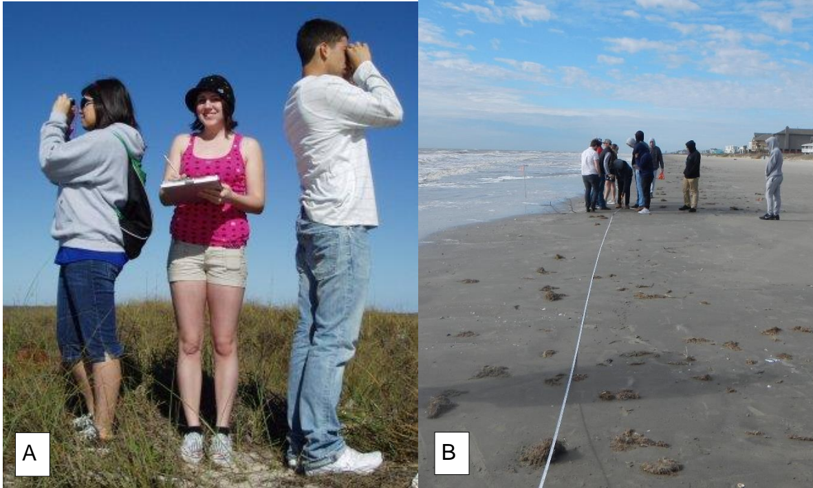
Figure 4. Students (A) using a sighting compass to measure dune orientation and (B) measuring how far along the shoreline the float (an orange) drifted to determine longshore current.
