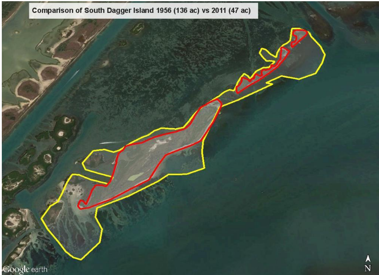
Figure 3. Comparison of the 1956 outline of Priority site 1 Southern Dagger Island (yellow) with the 2011 remnants of Dagger Island (red). In 1956 this section of Dagger Island was 136 acres in size, but now encompasses only 47 acres.
