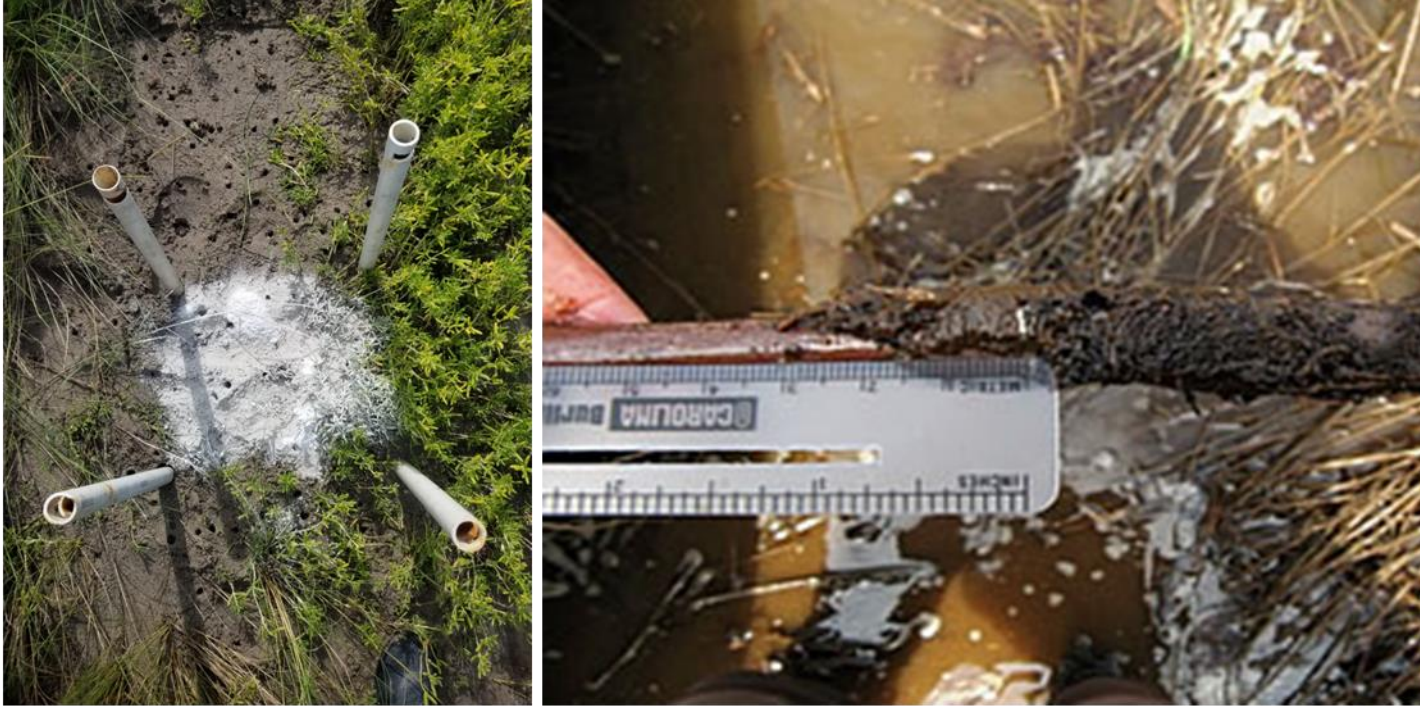
Figure 4a. (left) Feldspar set on the wetland surface as a marker horizon (PINS site). b. (right) a core showing sediment layers above the marker horizon (from: https://www.tidalmarshmonitoring.net/monitoring-methods-marker-horizons ).
