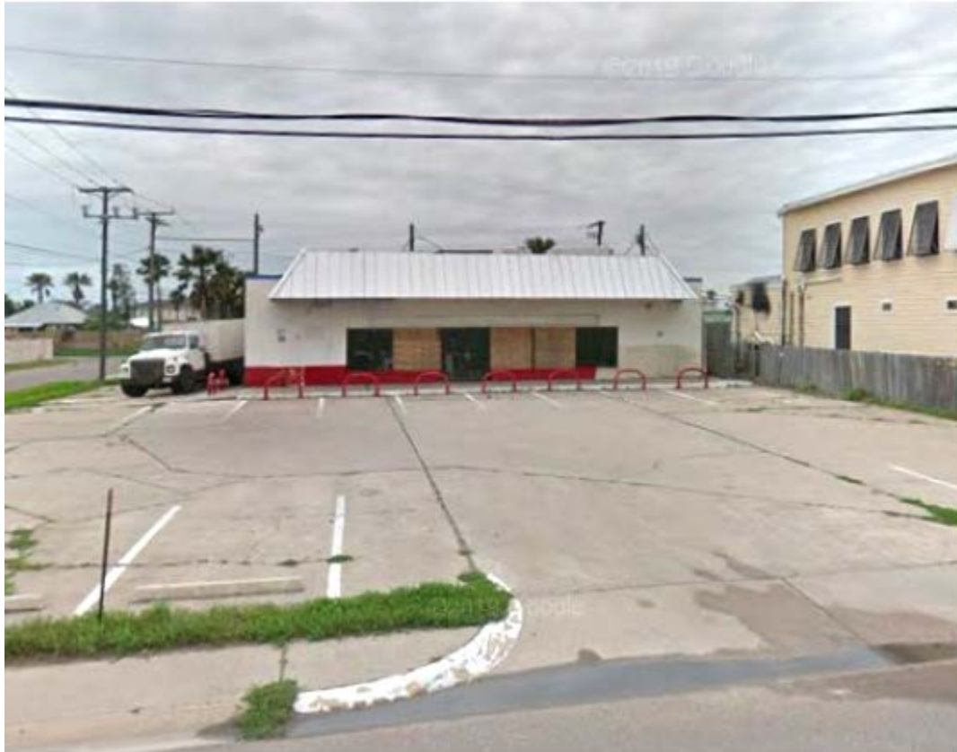
Even before Harvey, many businesses in Port Aransas covered their lots in concrete, contributing to nuisance flooding and runoff. Photo credit: Freese & Nichols.
