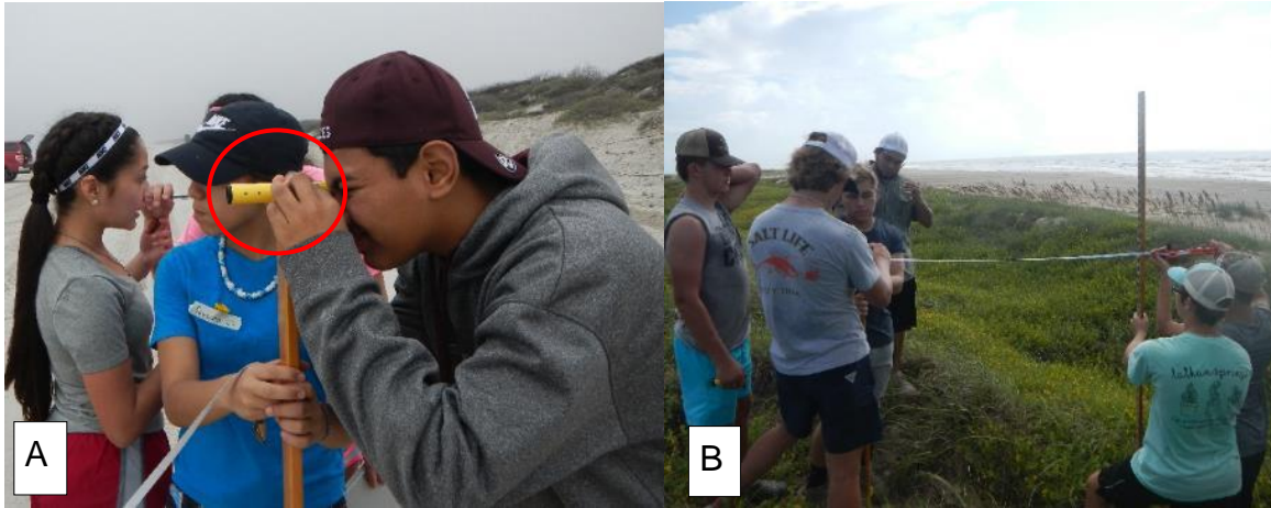
Figure 2. Students using (A) a sighting level to determine vertical offset between Emery rods and (B) a metric tape to measure horizontal distance.
