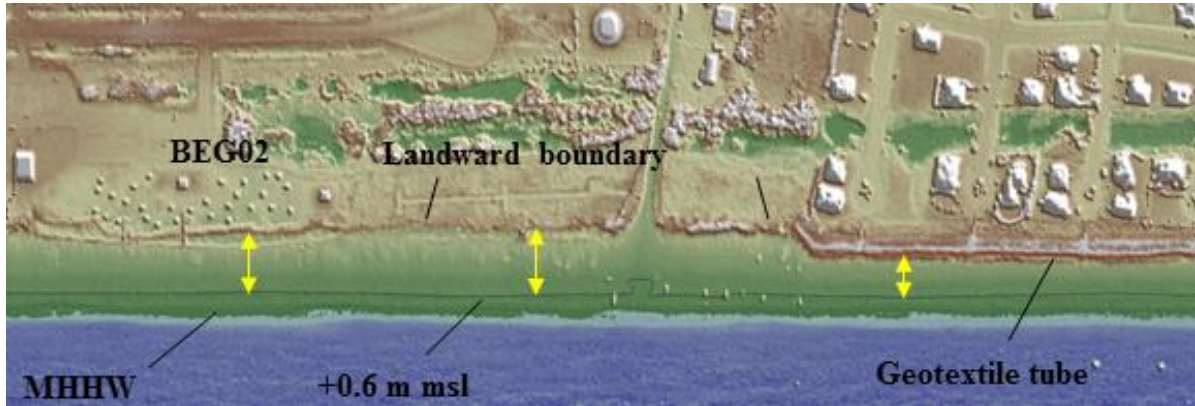
Figure 12. Lidar topographic-relief image of Galveston Island State Park and Pirates Beach subdivision. Note the difference in beach width between the natural beach and the area in front of the subdivision. From Gibeaut and others (2003).
