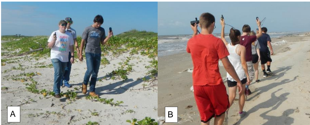
Figure 3. Students mapping (A) the vegetation line and (B) the shoreline (wet/dry line) using handheld GPS units.
