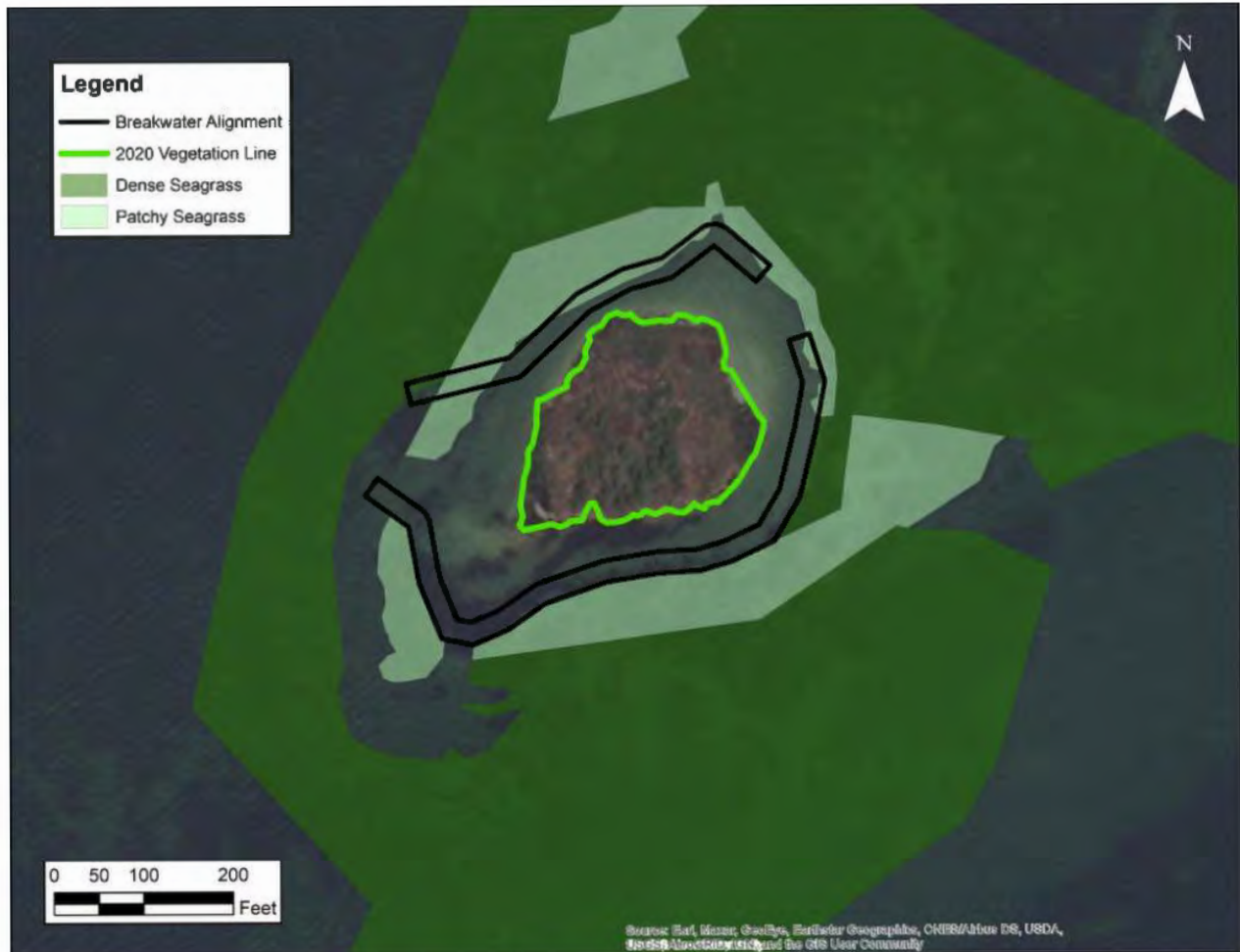
Figure 16. Plan view of Alternative 1: riprap breakwater
