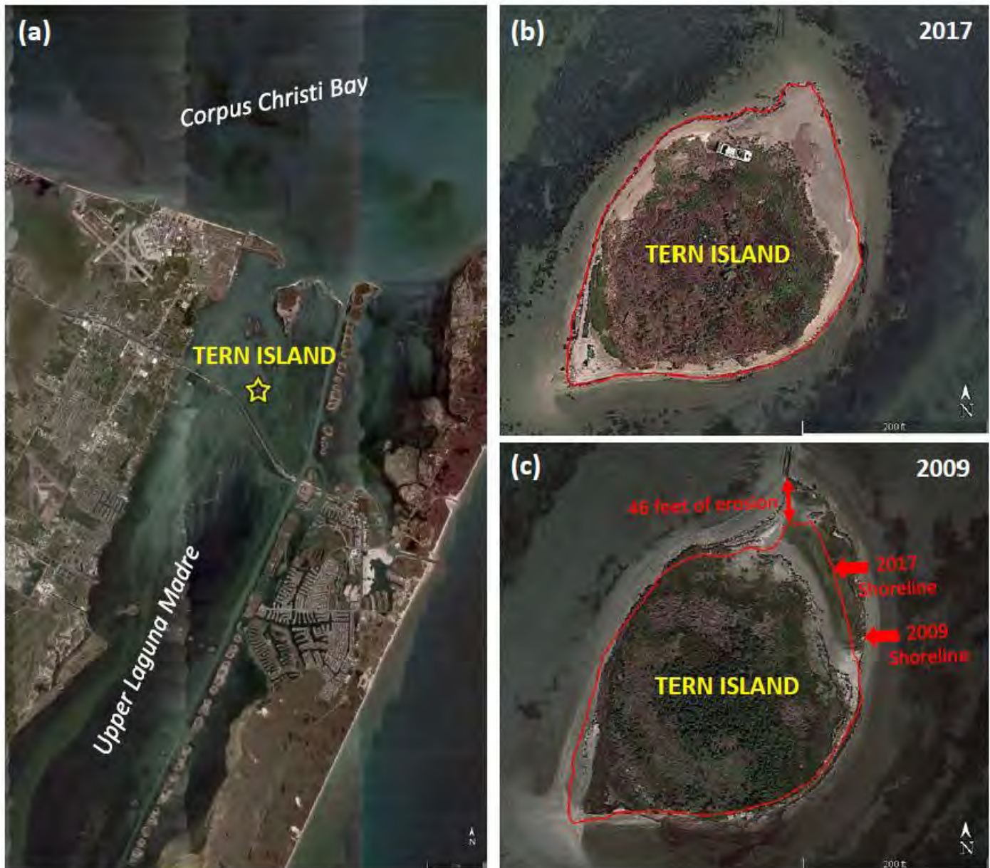
Figure 1. Vicinity map and aerial images of Tern Island depicting effects of erosion 2009 – 2017.
