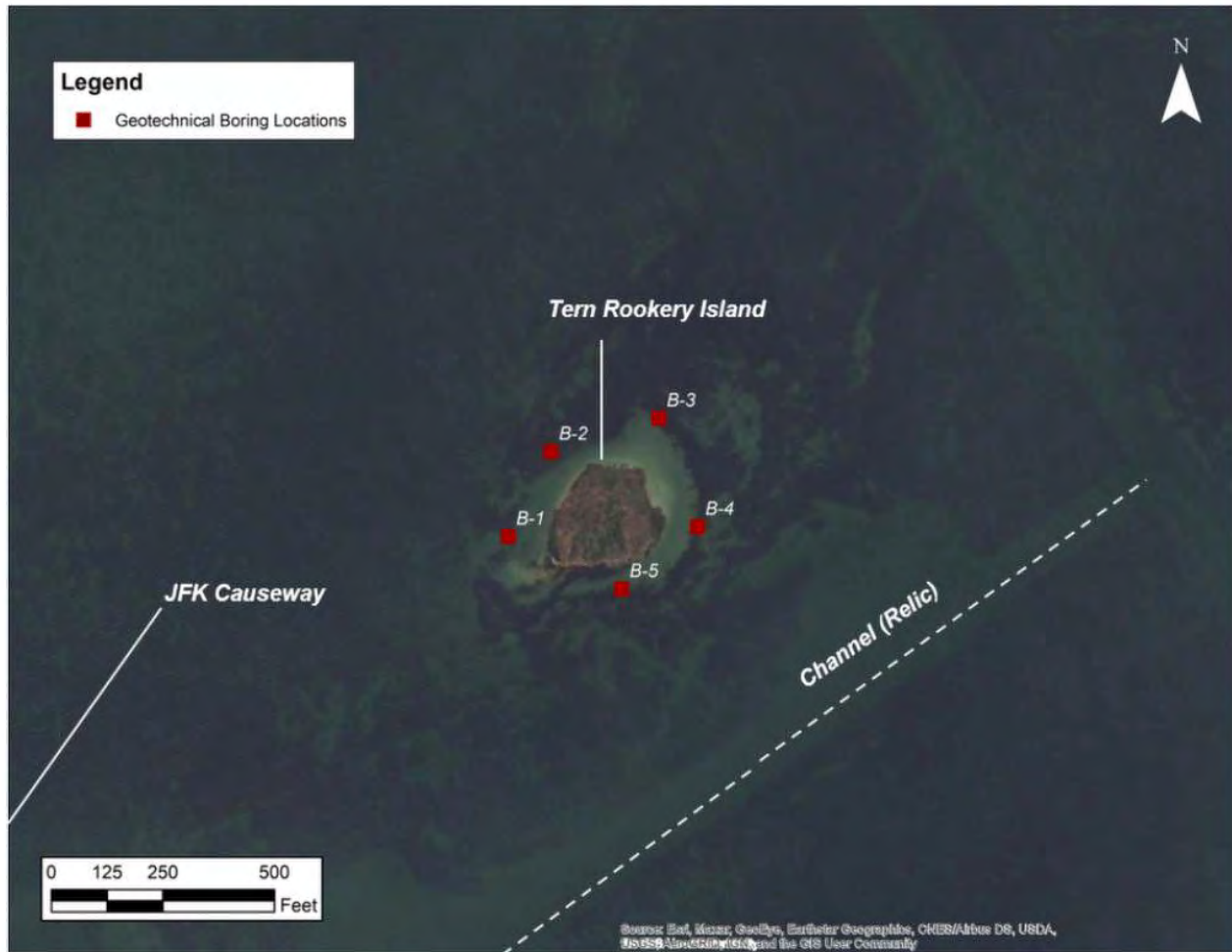
Figure 8. Geotechnical boring locations
