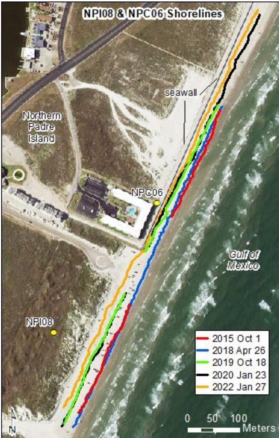
Figure 31. Shoreline position change between 2015 and 2022 along southern end of North Padre Island seawall and adjacent beach.
