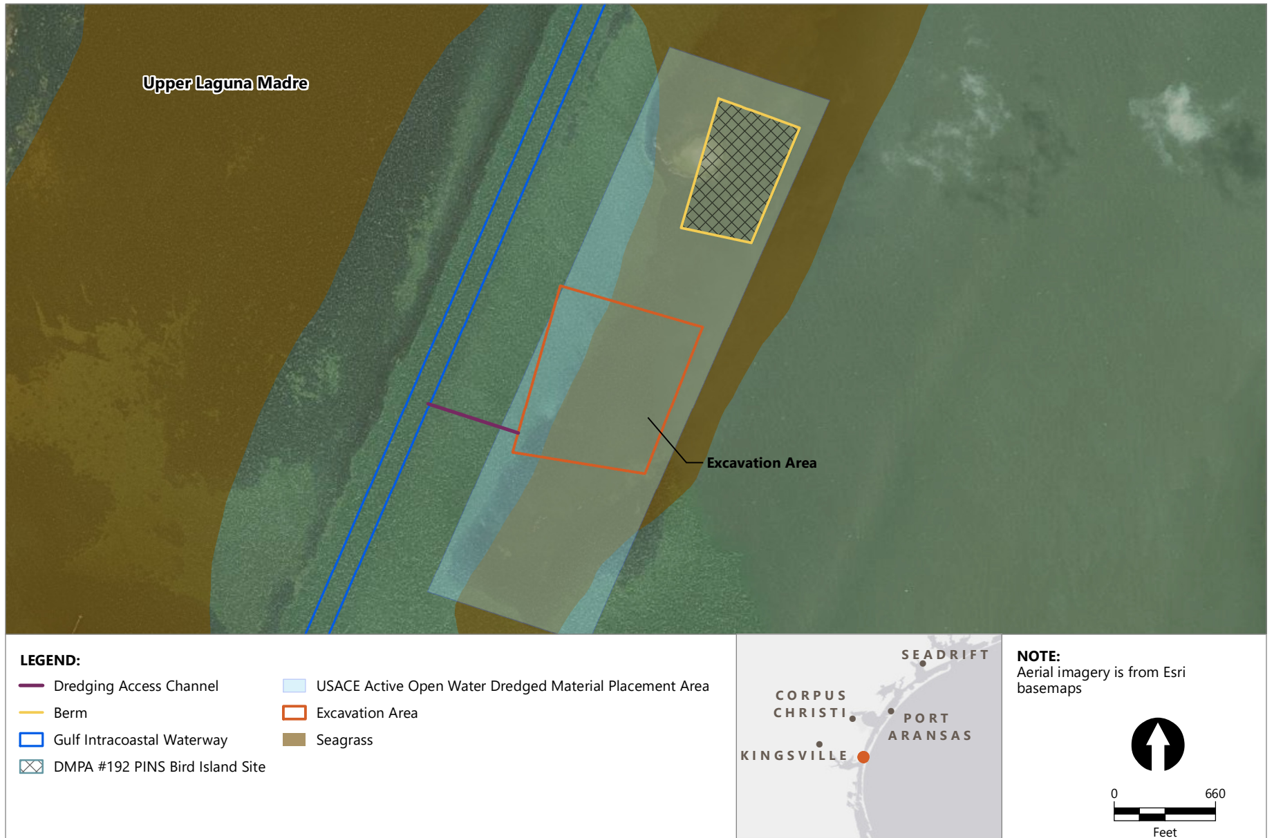
Figure 1 DMPA #192 PINS Bird Island Plan View DMPA #192 PINS Bird Island 10% Design Memorandum Texas Lower Coast Beneficial Use
