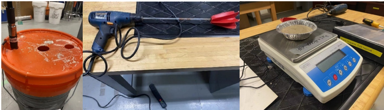
Figure 4.5: OBS calibration setup: OBS sensor submerged in turbulence chamber (left), power stirring device to generate turbulence in bucket (center) and incremental dry sediment quantity to be added (right).
