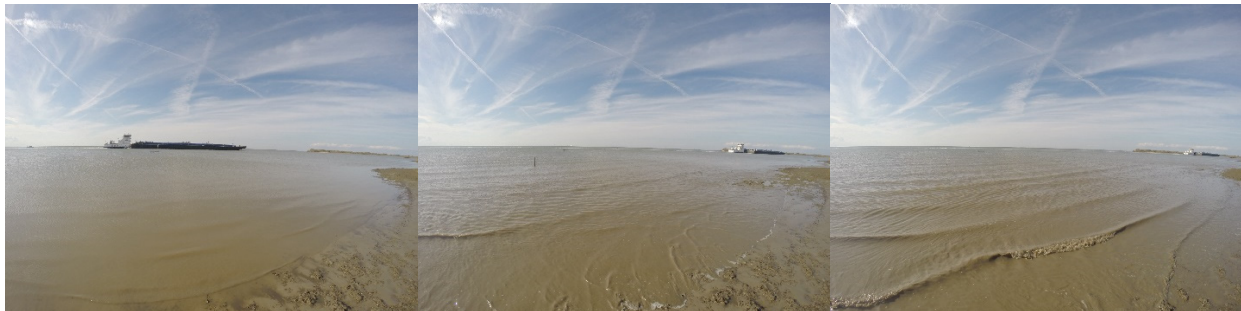
Figure 4.11: Sequence of photos (left to right) collected by GoPro camera mounted near the wetland edge of FS-3. The images clearly show the ship passage and ship wake patterns affecting the field site.
