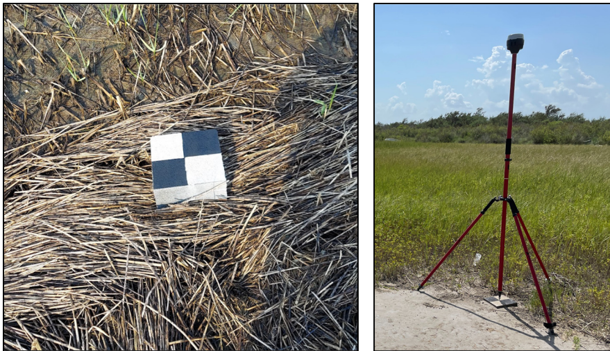
Figure 3.2: (left) Ground control point, (right) Setup for GNSS RTK receiver on GCP
