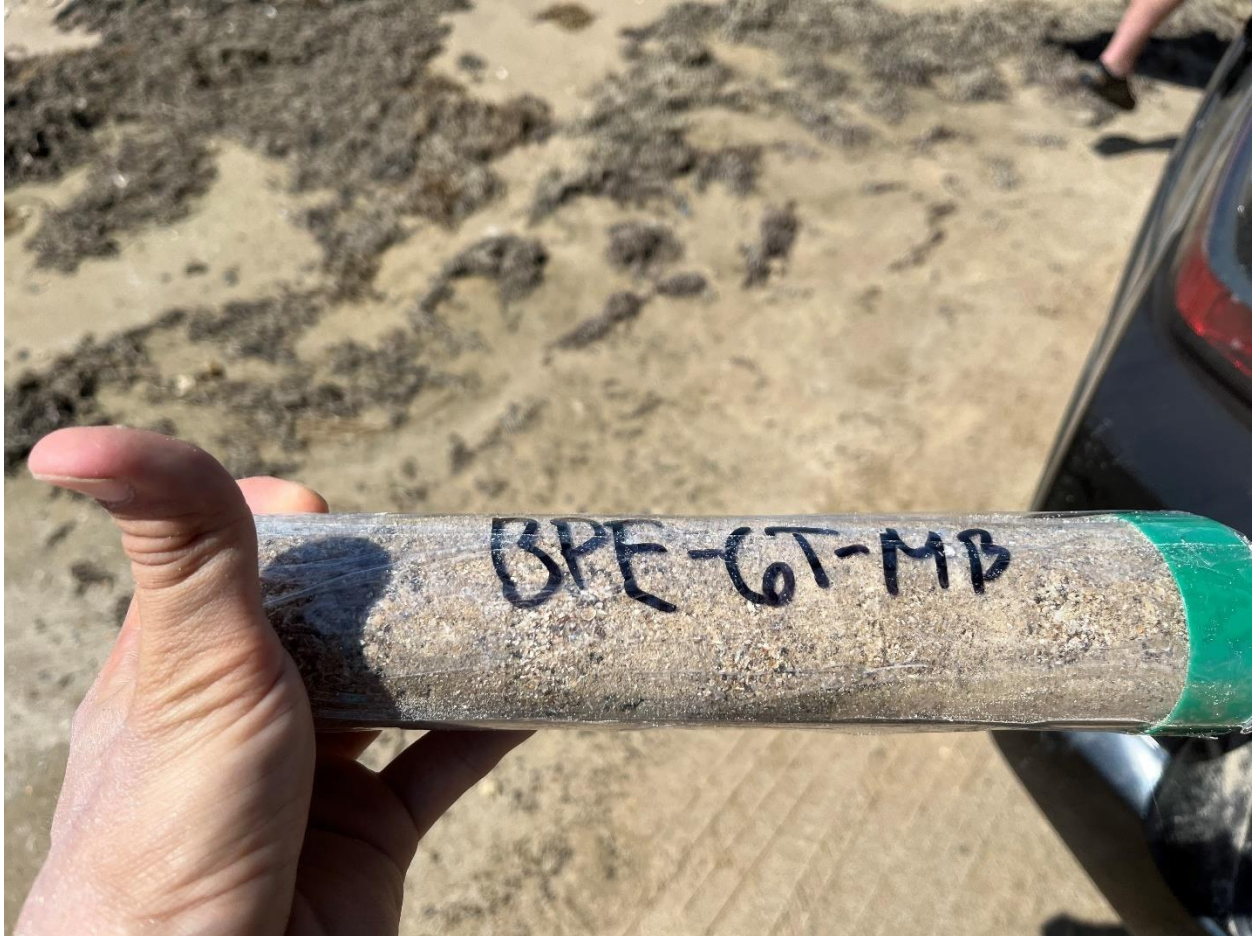
Figure 18. Sampling Tube 10" Long by 2" Diameter
