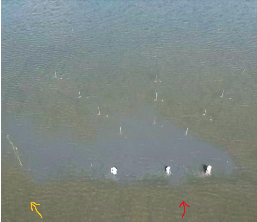
Plume begins to pull away from 1 st poles in all 3 directions and moves off towards the left.
