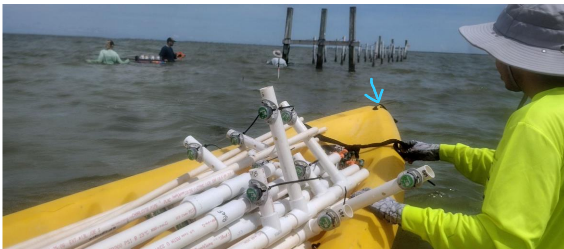
Deploying Light Loggers and Sediment Traps down-current of the cage line
