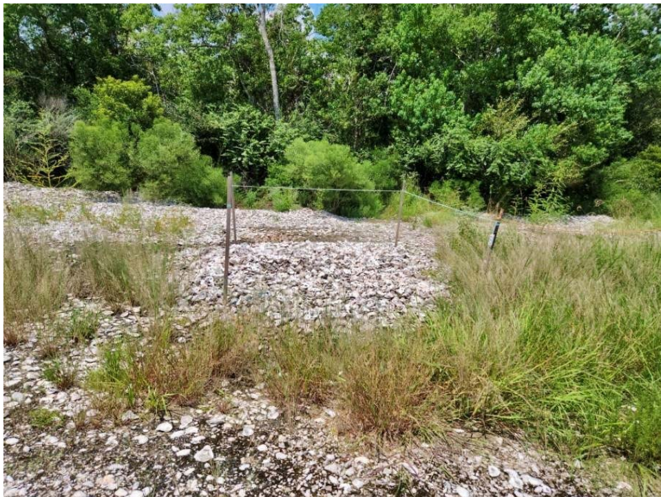
Figure 2. Assembled unfenced shell pile in preparation for sun curing experiment
