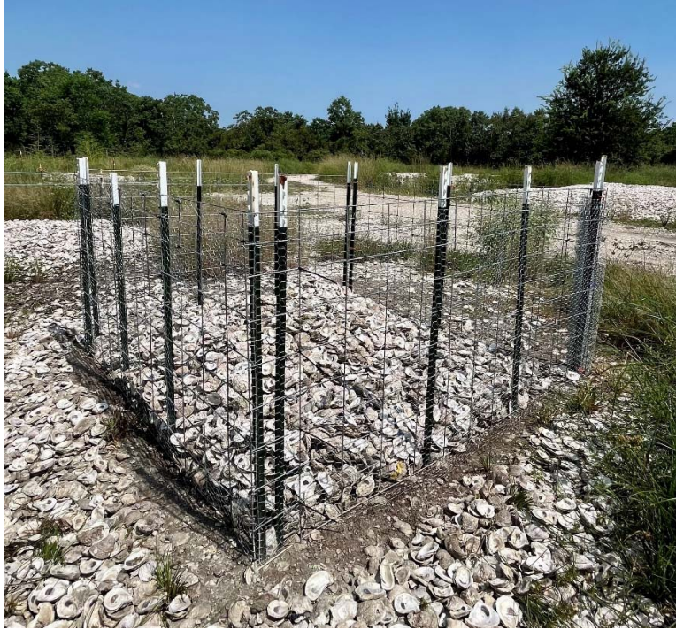
Figure 3. Assembled fenced shell pile (with chicken wire) in preparation for sun curing experiment
