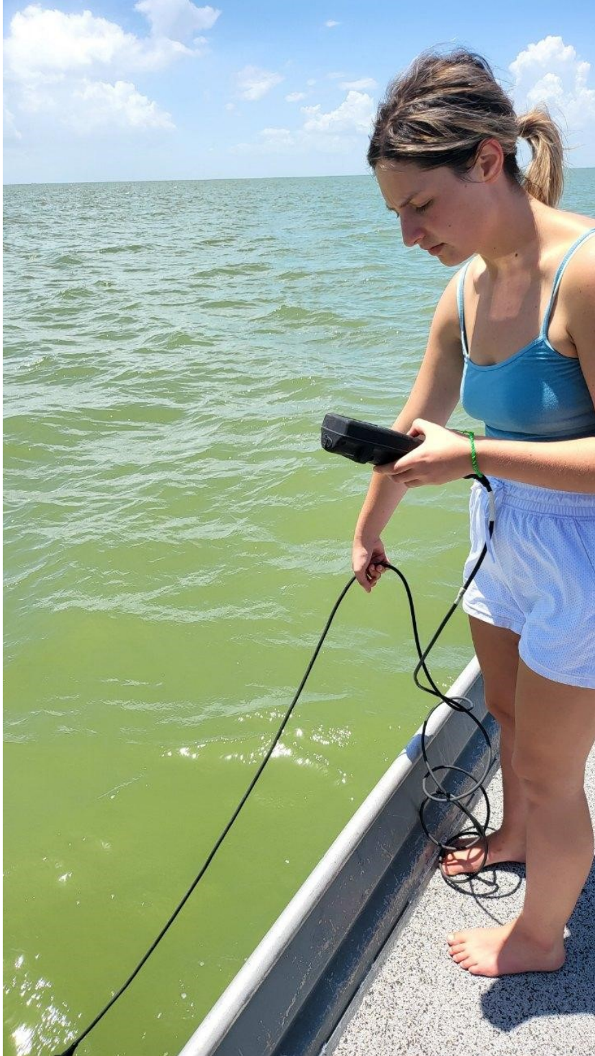
Figure 7: Collecting salinity and temperature observations using a Yellow Springs Instrument (YSI).
