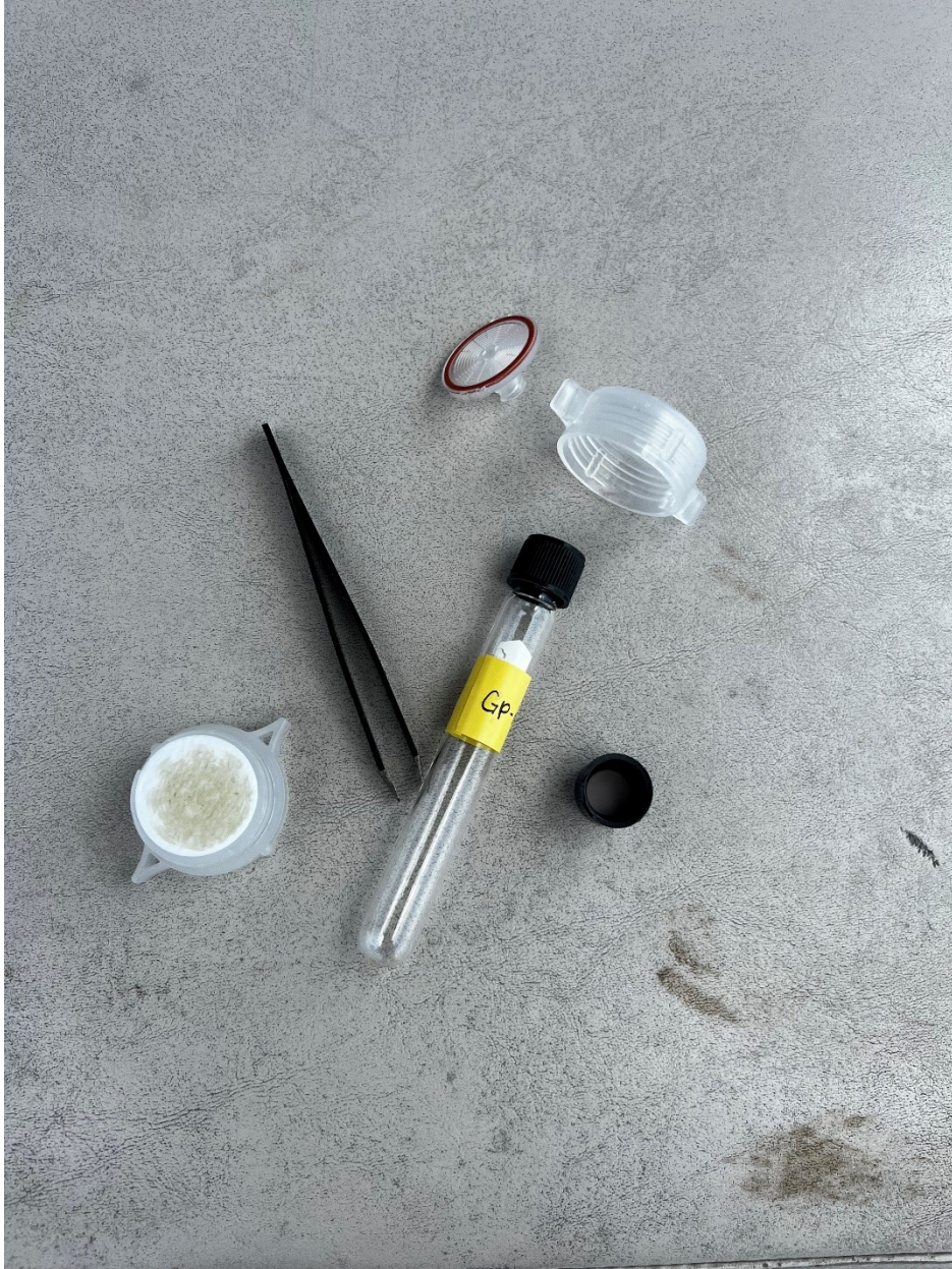
Figure 5: Equipment used to collect nutrient samples.
