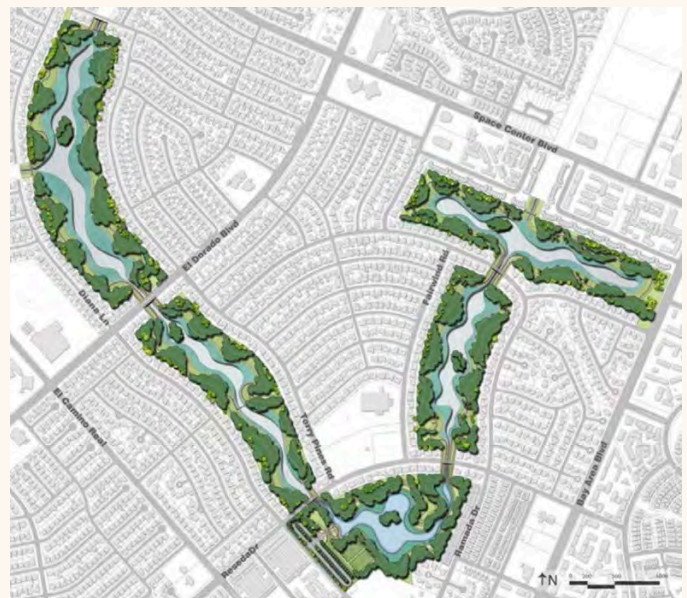
Figure 2: Design plans for Exploration Green Stormwater Wetland Park in Clear Lake, Texas. Image provided by CLCWA https://www.clcwa.org/_files/ugd/6e2815_68f51ebb41a0477eae7840083d27b9d.pdf
