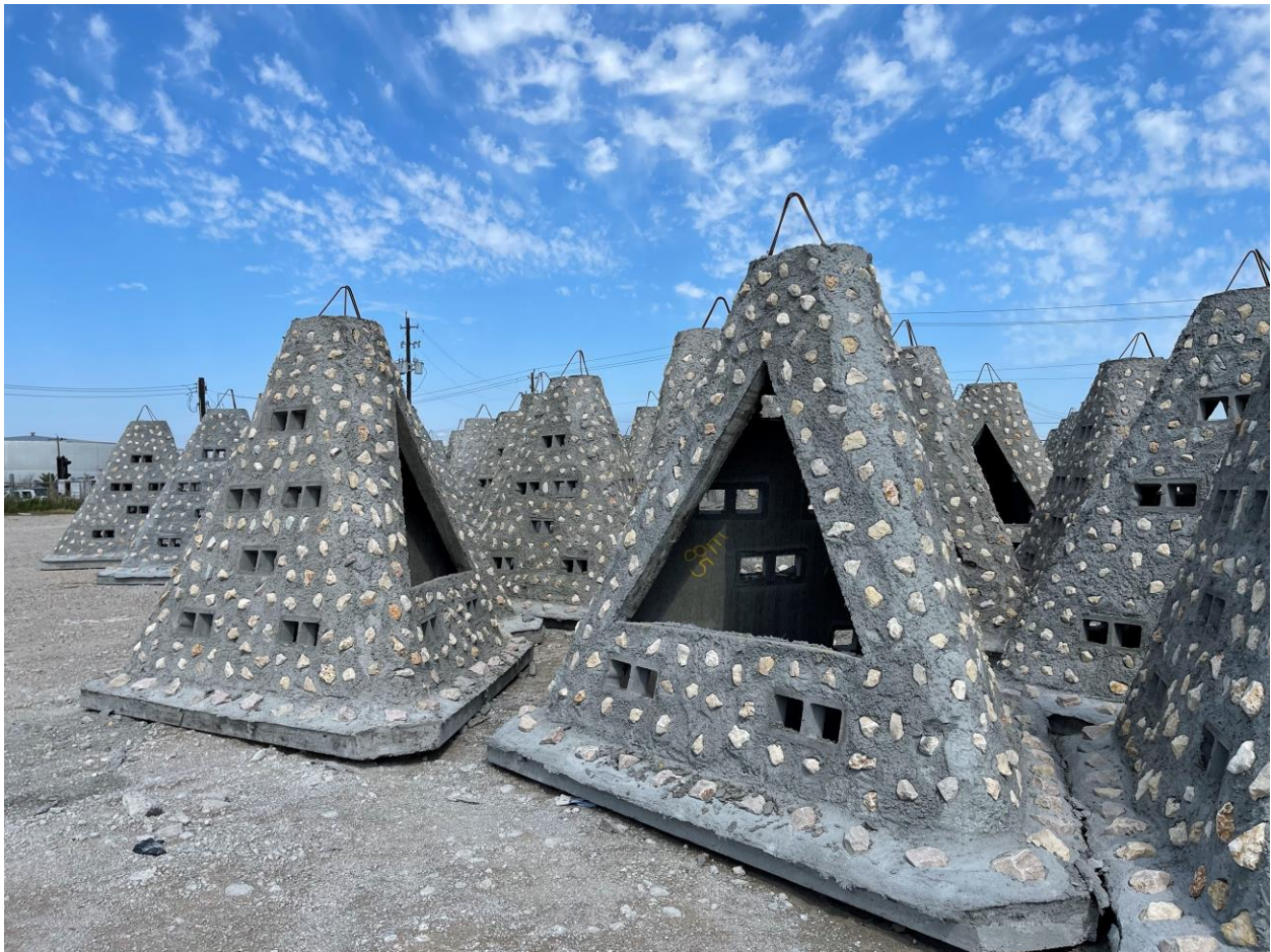
Figure 1. Mid-relief pyramids fabricated by Laredo in March 2022. Note the large opening that allows for escapement of marine life and prevents entanglement and entrapment. Also note the structurally complex surface, which allows encrusting organisms to recruit to the structures and maximize productivity.
