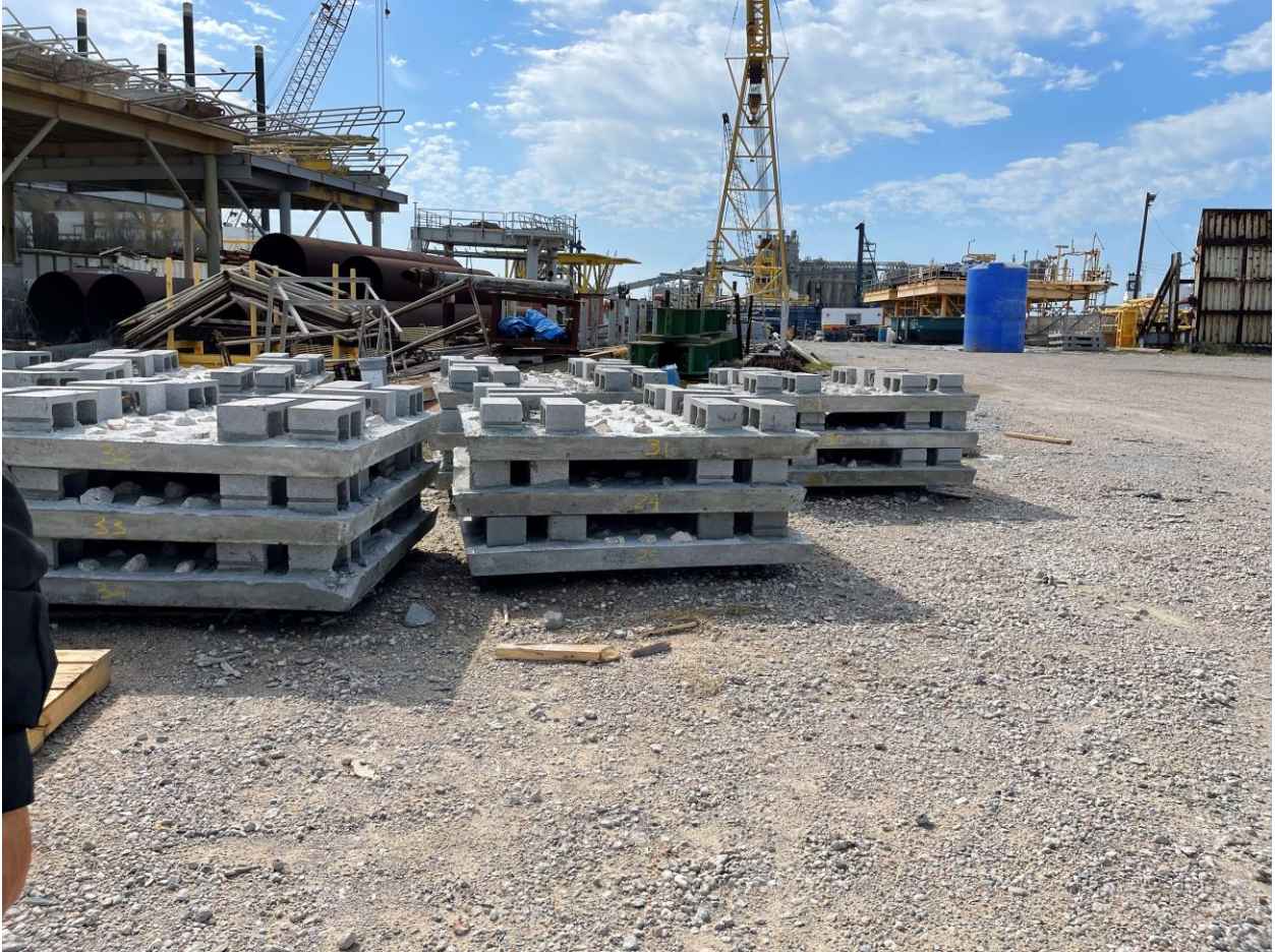
Figure 2. Low-relief plates fabricated by Laredo in March 2022. Note how vertical relief and structural complexity is increased when they are stacked.
