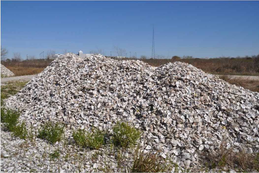
Figure 21. Cured oyster shell piled and consolidated at TX City Curing Site.
