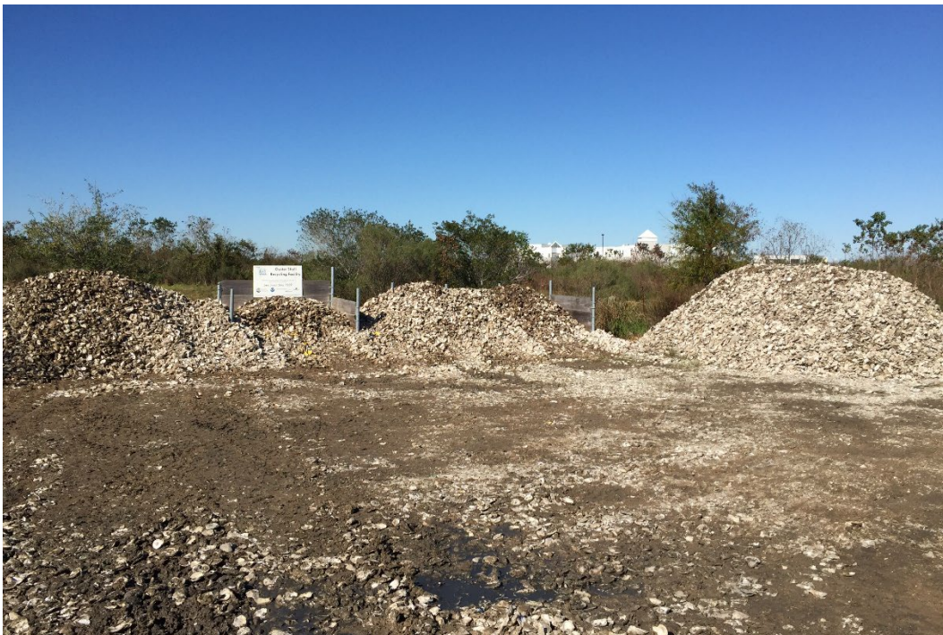
Figure 18. Recycled oyster shell piled for sun curing at TX City Curing Site.
