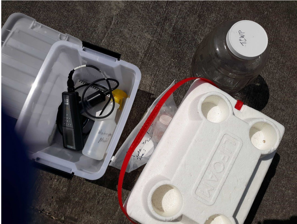
Figure 13 Sample collection supplies include a YSI handheld probe, a DI water spray bottle to rinse probes between samples, a field journal, a clean sampling jar, lab sample bottles in secondary containment Ziplock, and a cooler of ice.
