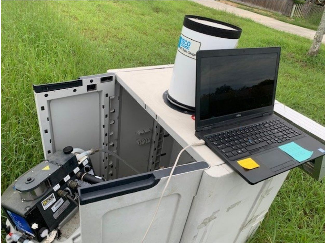
Figure 17 View of ISCO data port, rain gauge port, and battery port connections( from right to left) during a sample download.
