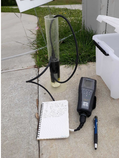
Figure 2: Water taken from sample collection and handheld data being recorded at Exploration Green Phase 4.
