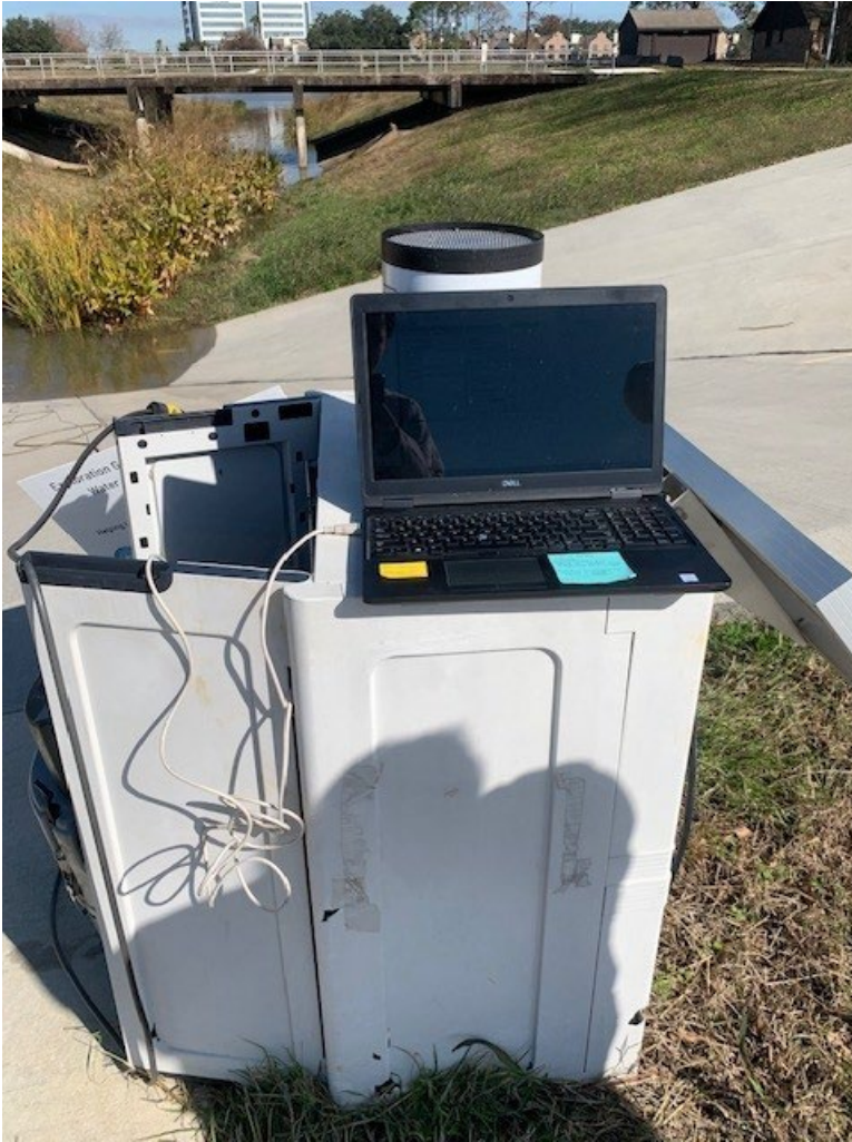
Figure 16 Laptop connected to ISCO data port for download at Phase 1.
