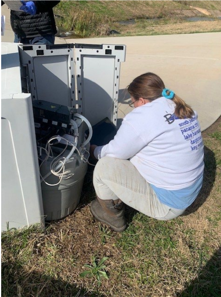
Figure 15 Christie is downloading quarterly rainfall and flow levels from ISCO samplers after third quarter in December 2023.
