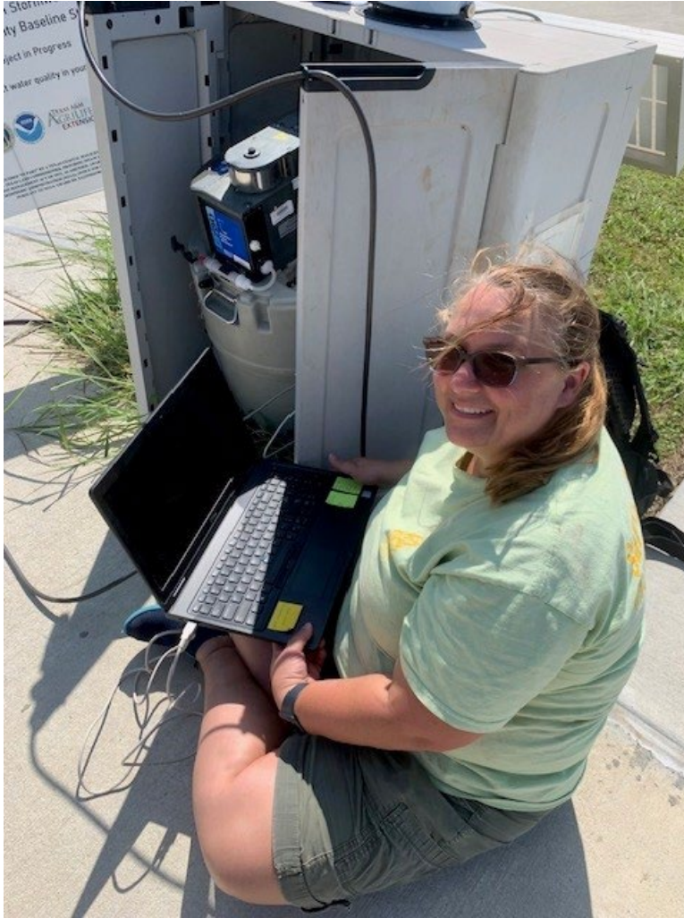
Figure 14 Christie downloading passive rainfall and flow meter data from sampler after the first quarter in July 2023.
