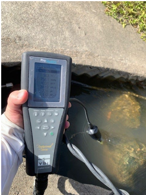
Figure 3: Handheld water sample being collected on a non-lab sample day at Phase 1 outfall.
