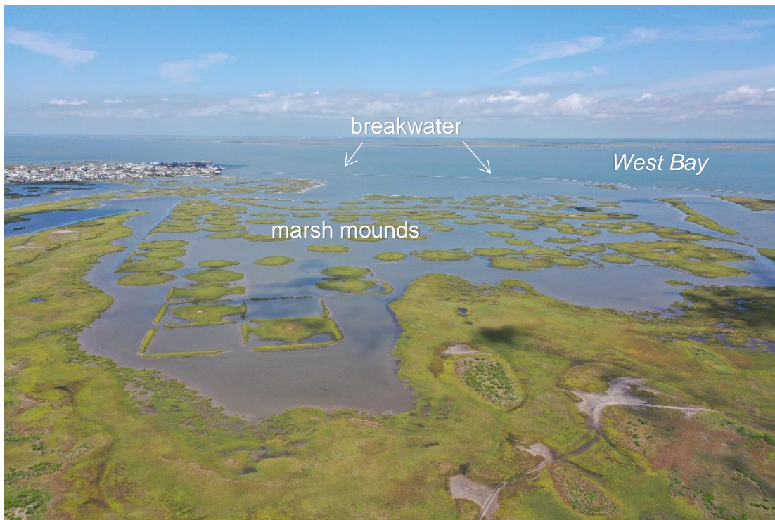
Figure 8. Marsh restoration projects along the West Bay shoreline of Galveston Island State Park.
